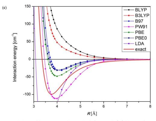
**Figure 1.** (a)The step of determining crystal structure by the first principles [35]. (b) Density functional theory combined with various theoretical methods. (c) Performance comparison of argon dimer by different DFT methods. The datum curve [36] is accurate to its line width. The acronyms define various DFT methods, for example, see Reference [37]. Reprinted (adapted) with permission from Ref. [35]. Copyright 2014, American Chemical Society.
