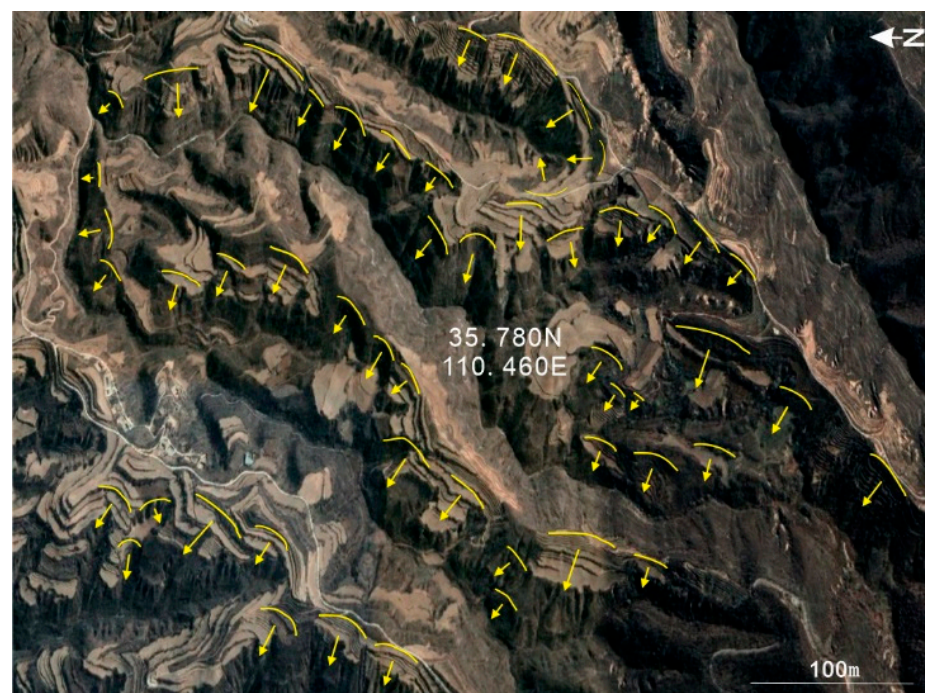
Figure 7. Landslide cluster map in the study area. (the yellow arrows in the figure indicate the direction of the landslide).
