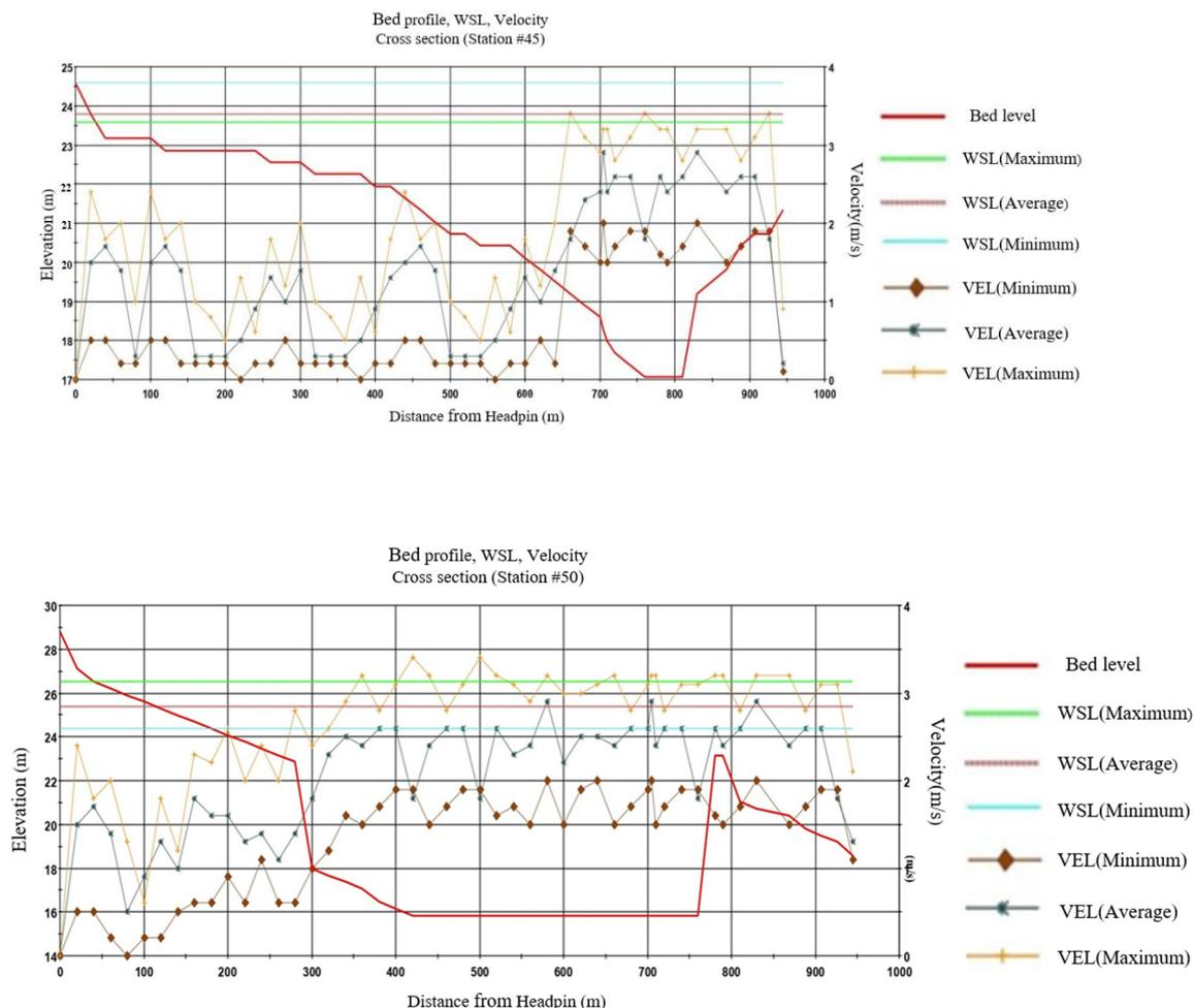
Figure 5. Velocity profile of sampling stations #45 and #50.
