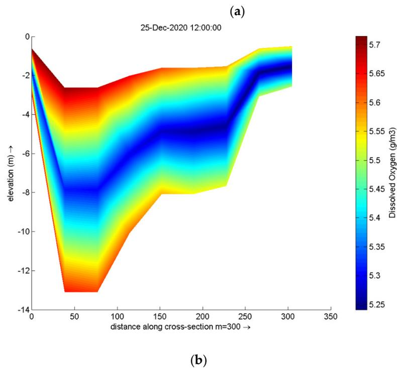
**Figure 10.** (a) Location of the cross section for sampling point #47. (b) Dissolved oxygen concentration for sampling point #47.
