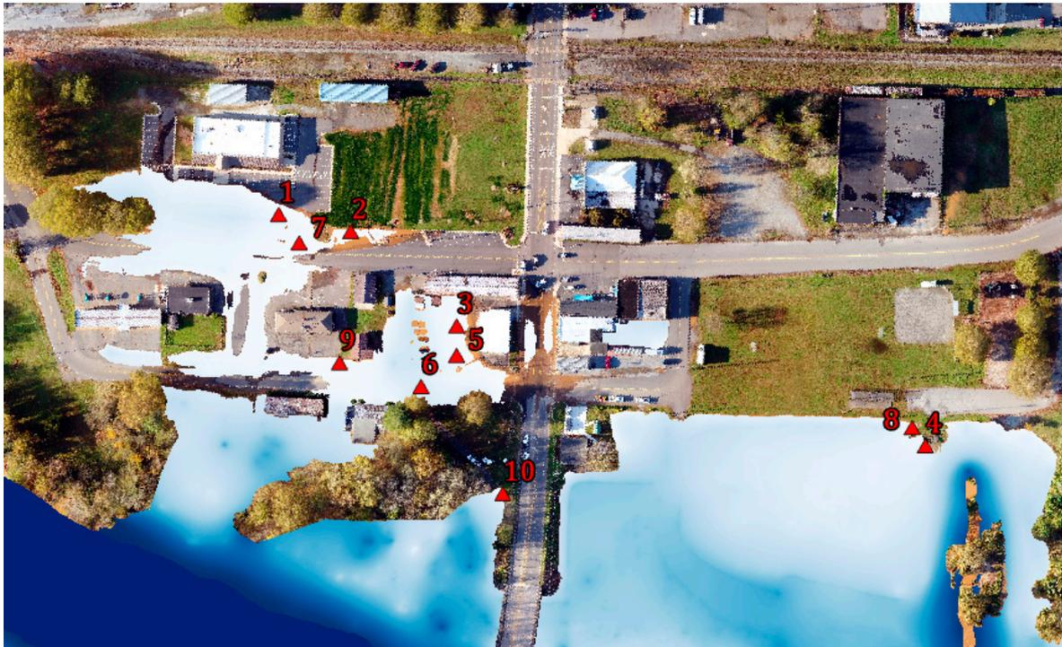
**Figure 10.** Floodwater depth measurement locations for depth model validation.
