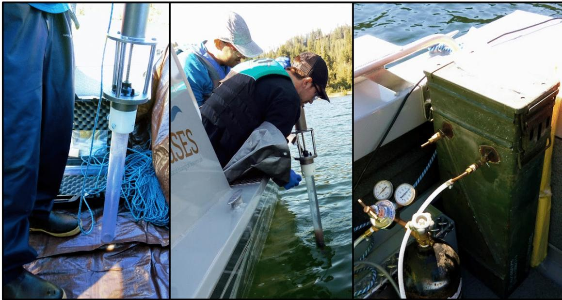
**Figure 4.** Kajak–Brinkhurst gravity corer, free fall use from the University of Idaho Lake Social Ecological Systems boat in Coeur d’Alene Lake, and storage of the cores in the gas-tight containers with an N<sub>2</sub> source for atmosphere flushing.
