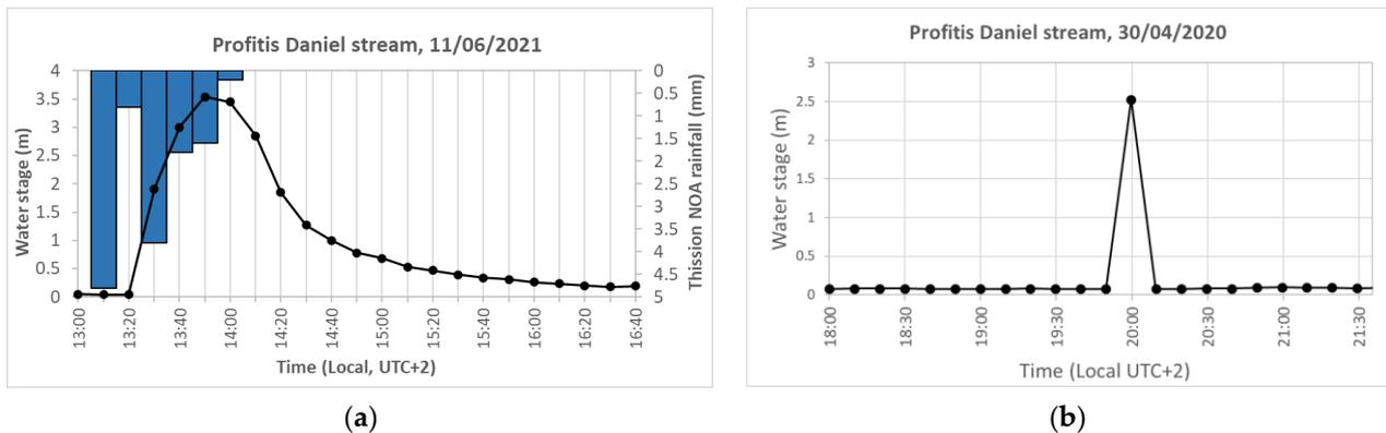
**Figure 5.** Hydrographs flagged with “warning” in two cases of abrupt water stage changes 10 min time at Prophitis Daniel station exhibiting: (a) an actual hydrograph: increase by 1.9 m and (b) a spontaneous error in measurement. Blue bars indicate rainfall, lines with dots indicate water stage.
