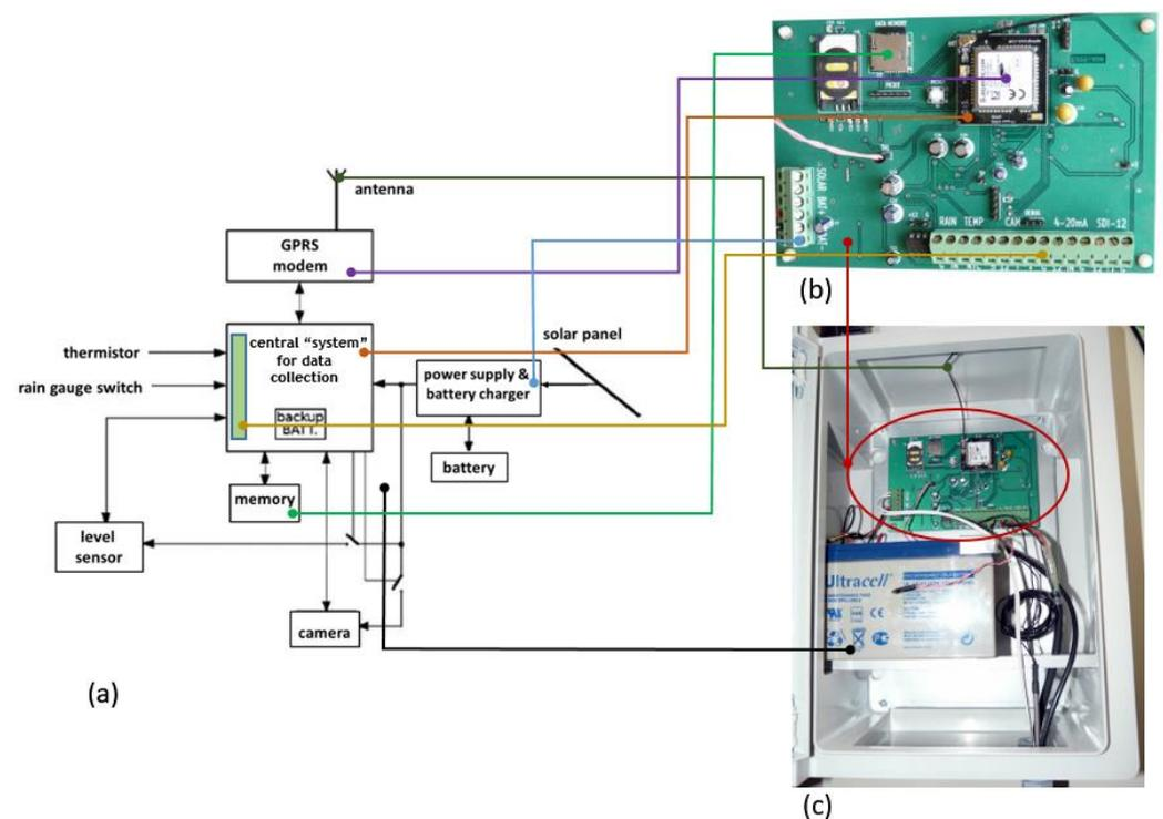
**Figure 8.** HYDRONET station: (a) block diagram, (b) control board, and (c) box interior.
