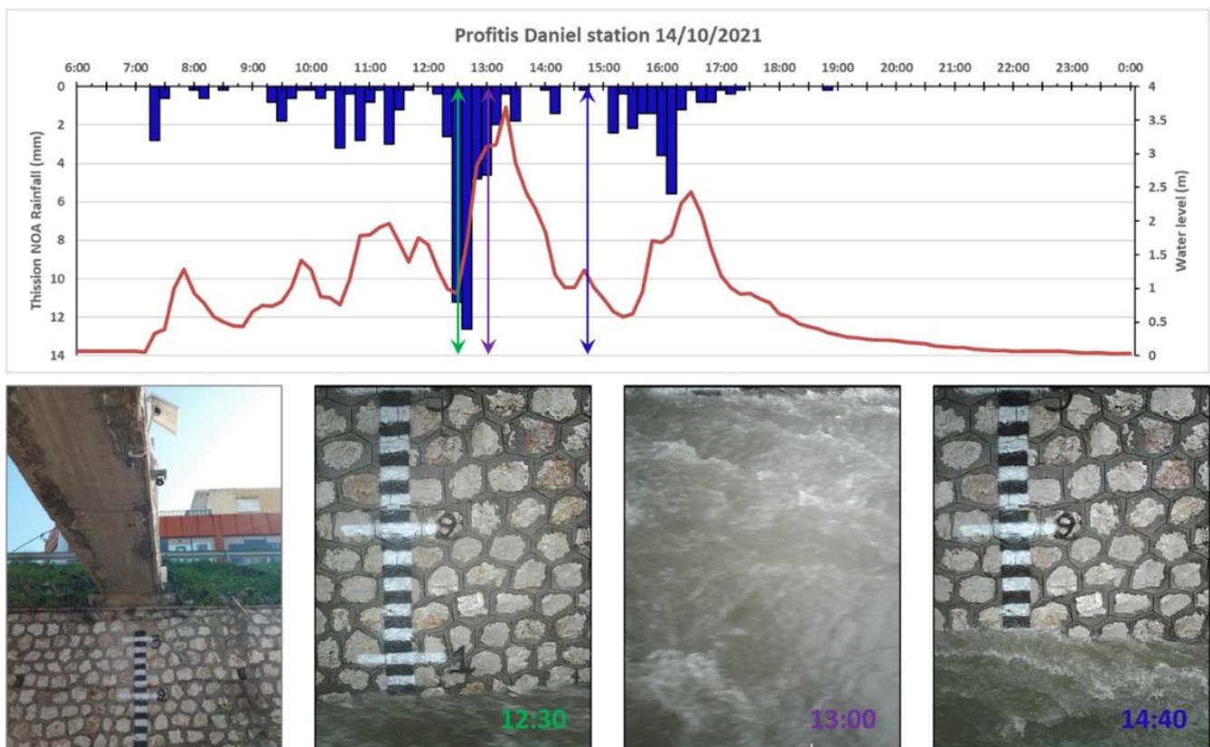
**Figure 9.** Profitis Daniel HTM station. Rainfall (blue bars) and hydrograph (red line) on 14 October 2021 (**upper part**)—the arrows indicate the stage at the time of the photos in the lower part. (**Lower part**) shows a picture of the station (**left**) and consecutive photos captured automatically by the station's camera, exhibiting the flow conditions in the stream. Rainfall data are from the automatic actinometric–meteorological station of IERSD/NOA at Thission.
