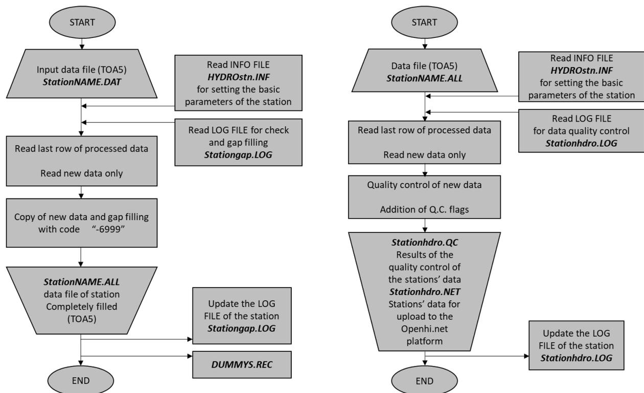
**Figure 4.** Block diagrams: (left) Diagram of the process of checking and filling in gaps and (right) diagram of the procedure for quality control of the data.
