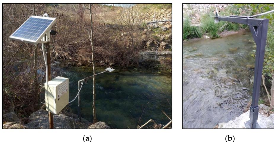
**Figure 3.** HTM Evrotas station: (a) installation on the right bank of the river looking downstream, and (b) close-up photo of the sensor assembly.
