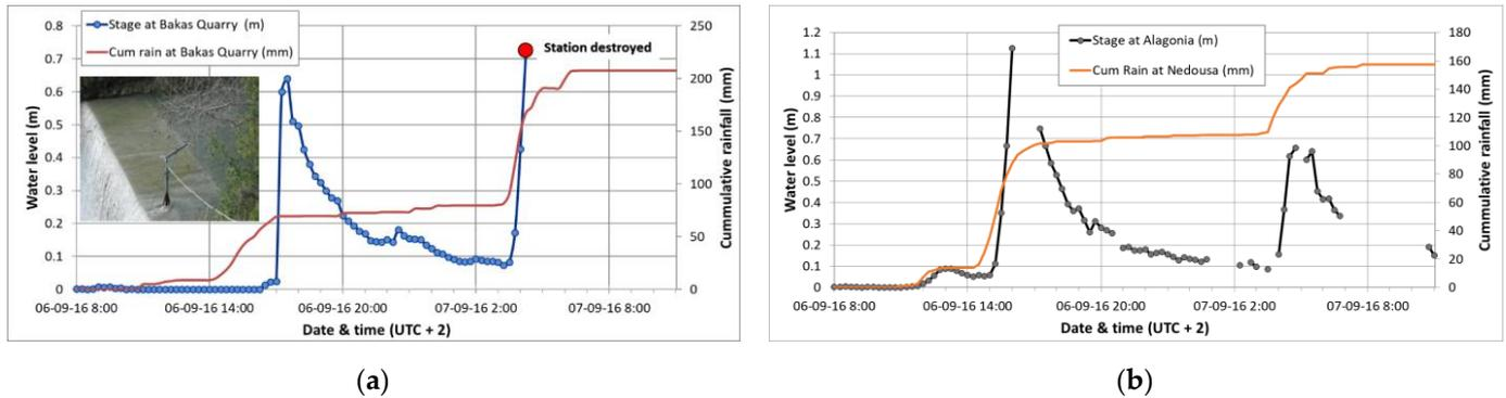
Figure 10. September 2016 flood at Baka's Quarry station (inset) (a) and at Alagonia station (b).
