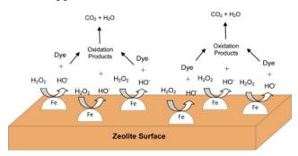
**Figure 2.** Formation of radicals on Fe-zeolite during oxidation of textile dyes. Reproduced with permission from Queirós et al., heterogeneous Fenton reaction oxidation using Fe/ZSM-5 as catalyst in a continuous stirred tank reactor, published by Separation and Purification Technology, 2015 [25].
