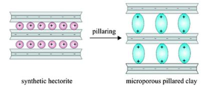
**Figure 1.** Pillaring, exchange of simple cations for polyoxo cations, e.g., Al-Fe polycation  $(Al_{13-x}/Fe_x)^{7+}$ , see Muñoz et al. [30]. Reproduced with permission from Stöcker et al., realization of truly microporous pillared clays, published by Chemical Communications, 2018 [31].
