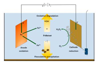
Figure 3. Electro-Fenton reaction mechanism diagram [42].
