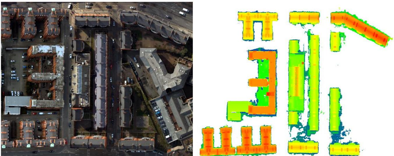
Figure 17. Regional reconstructed orthophoto and point cloud.
