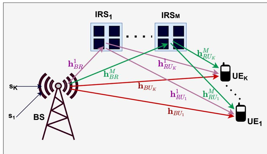
Figure 10. IRS-assisted Downlink Communication System: Multi-IRS and Multi-User.
