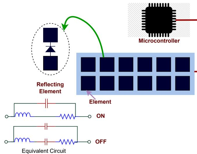
**Figure 1.** Basic architecture of IRS [6].
