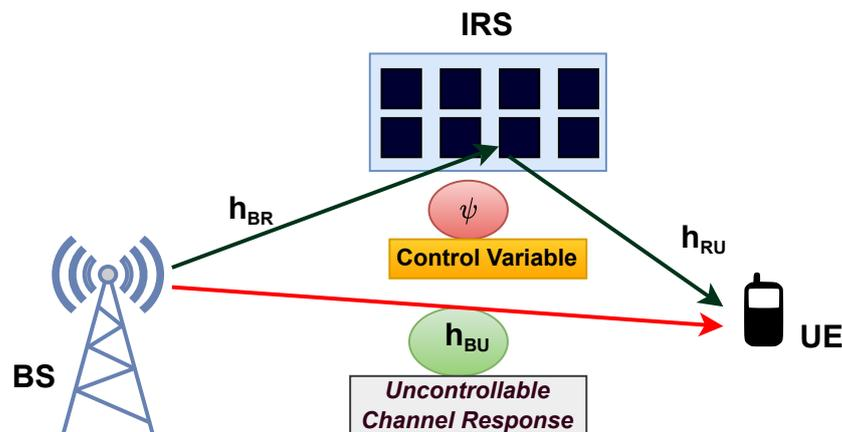
Figure 8. IRS-assisted Communication System: Single IRS and Single User.
