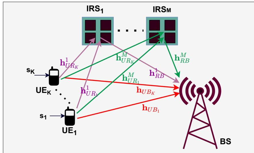
Figure 9. IRS-assisted Uplink Communication System: Multi-IRS and Multi-User.
