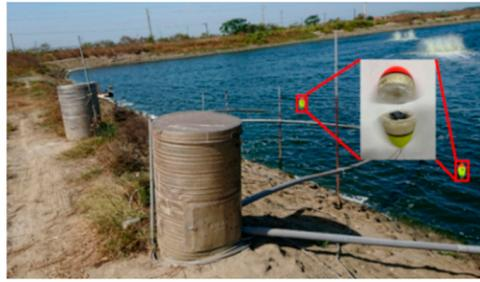
Figure 14. The buoy is placed in the breeding pond.
