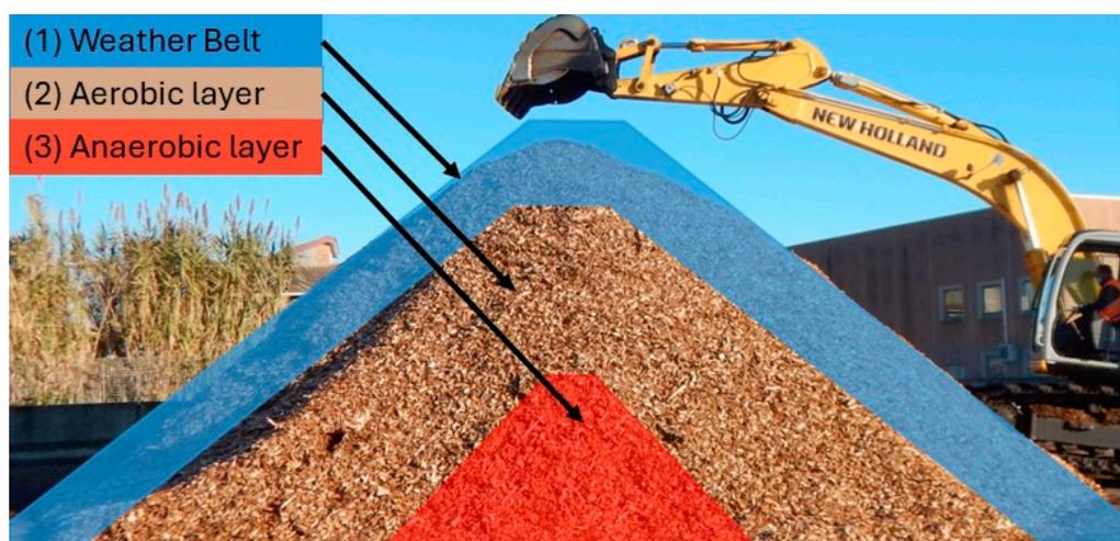
**Figure 4.** Model of the vertical profile of a woodchip pile after open-air storage according to [17].
