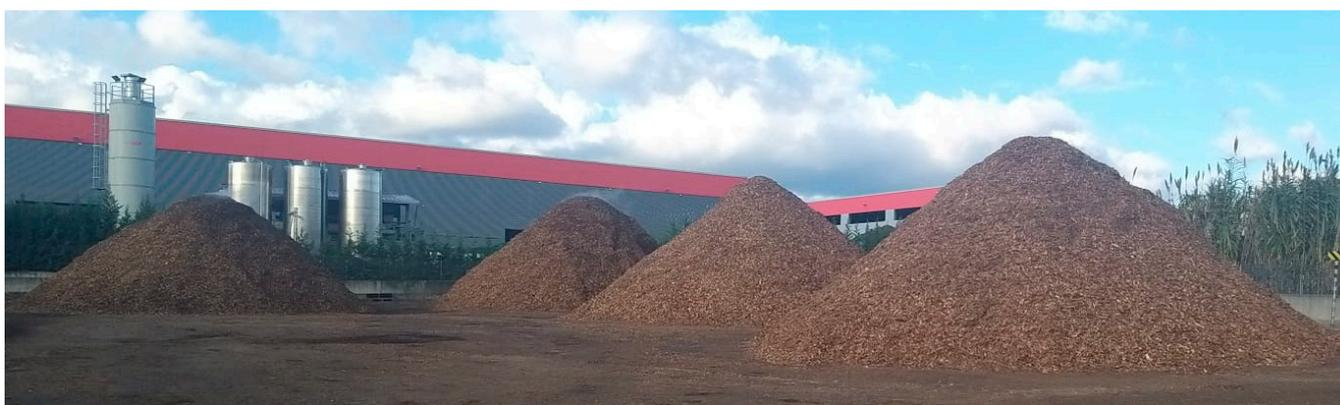
**Figure 1.** Layout of the test piles just after their construction. The wet biomass composing the two piles in the background is already steaming, while the two dry piles in the forefront show no sign of heat development.
