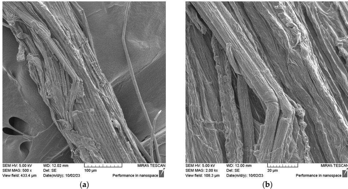
**Figure 6.** SEM micrographs of barley fiber isolated from the straw of the REX variety from 2021: (a) technical fiber under magnification of 500 $\times$  and (b) the ultimate fiber as part of the technical fiber under magnification of 2000 $\times$ .
