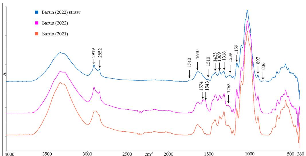
**Figure 12.** FTIR spectra of barley fibers isolated from straw of the new Barun variety.
