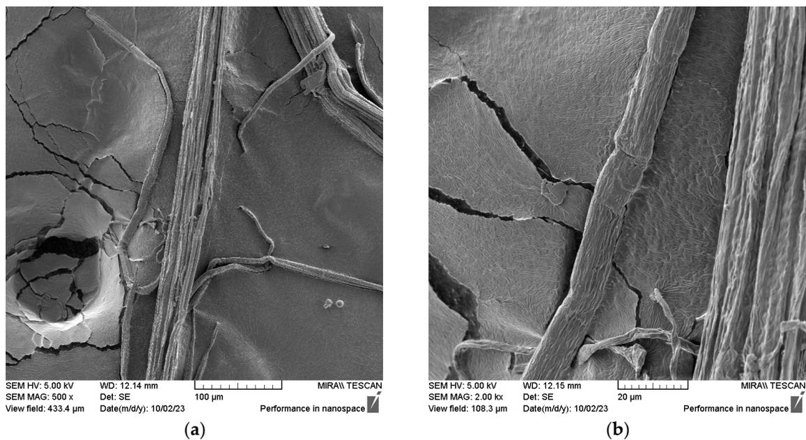
**Figure 8.** SEM micrographs of barley fiber isolated from the straw of the Barun variety from 2021: (a) technical fiber under magnification of 500 $\times$  and (b) the ultimate fiber as part of the technical fiber under magnification of 2000 $\times$ .
