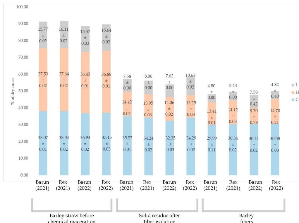
**Figure 10.** Chemical composition of barley straw before chemical maceration, solid residue after fiber isolation, and barley fibers, where L is the lignin content (wt.%), H is the hemicellulose content (wt.%), and C is the cellulose content (wt.%).
