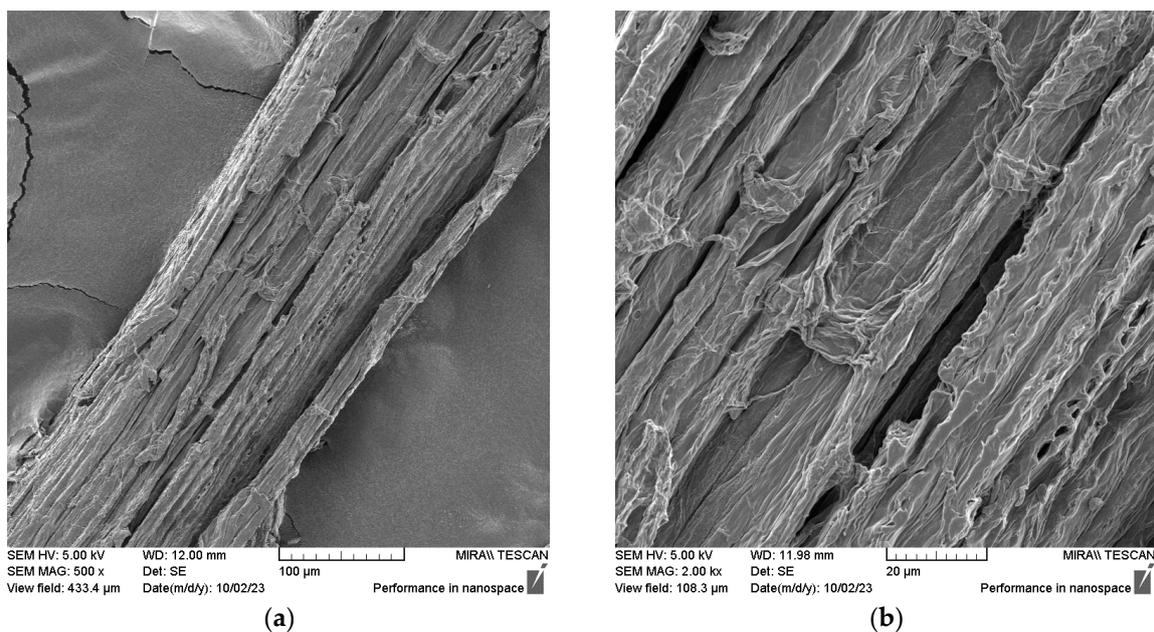
**Figure 7.** SEM micrographs of barley fiber isolated from the straw of the REX variety from 2022: (a) technical fiber under magnification of 500 $\times$  (b) the ultimate fiber as part of the technical fiber under magnification of 2000 $\times$ .
