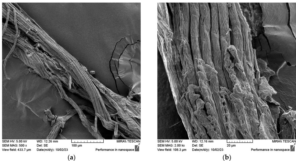
**Figure 9.** SEM micrographs of barley fiber isolated from the straw of the Barun variety from 2022: (a) technical fiber under magnification of 500 $\times$  and (b) the ultimate fiber as part of the technical fiber under magnification of 2000 $\times$ .
