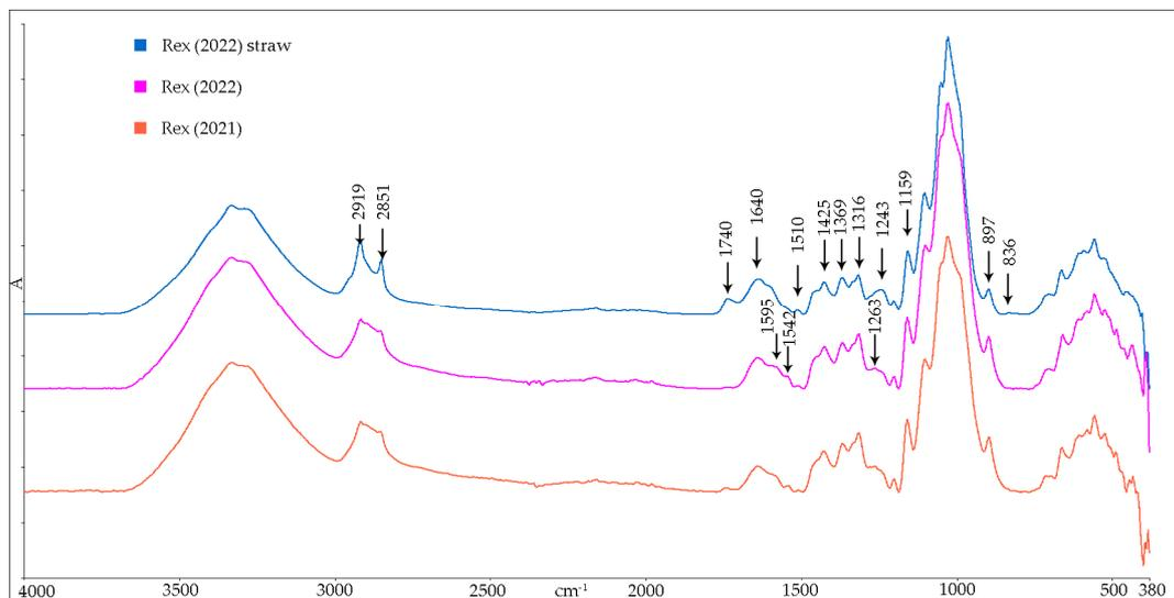
**Figure 11.** FTIR spectra of barley fibers isolated from straw of the old Rex variety.
