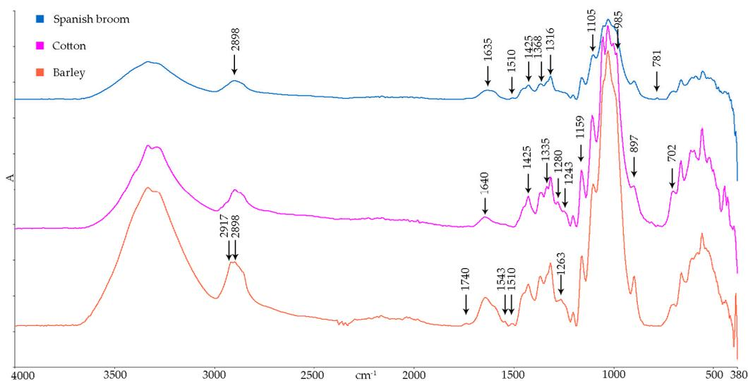
Figure 13. FTIR spectra of barley fibers compared to Spanish broom and cotton fibers.
