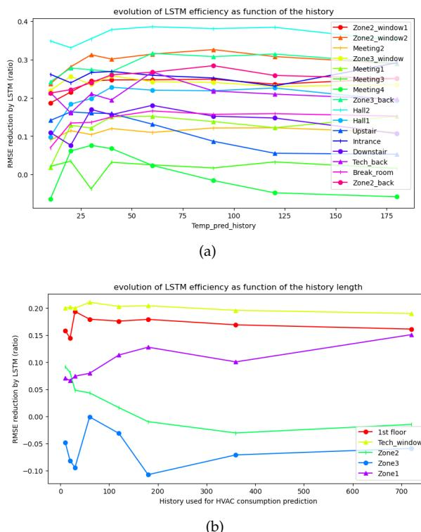
**Figure 5.** Study of performances as a function of history length in minutes. (a) Temperature forecasting performances; (b) HVAC consumption forecasting performance.
