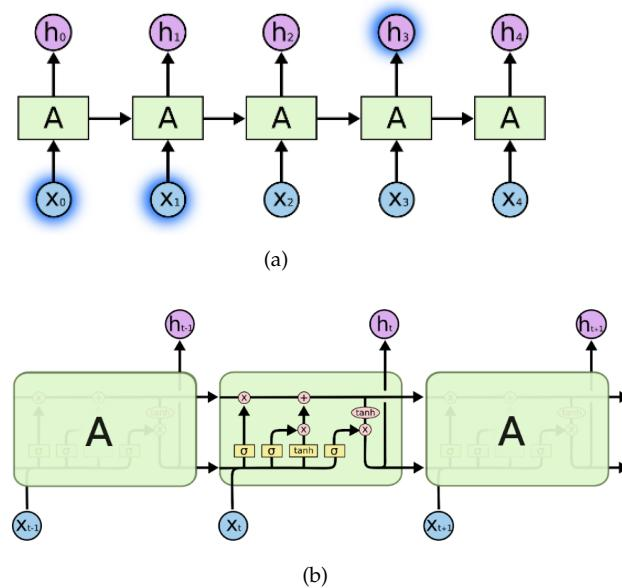
**Figure 2.** LSTM Neural Network principle and architecture. (a) LSTM principle; (b) LSTM architecture.
