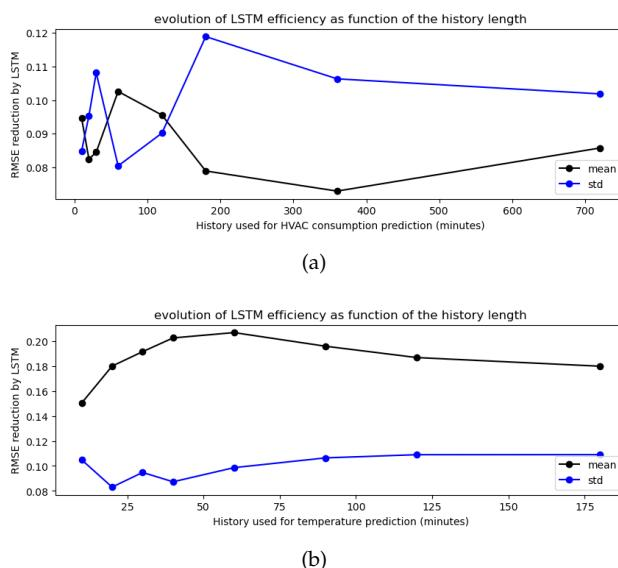
**Figure 6.** Study of performances as a function of history length. (a) Consumption forecasting performances; (b) temperature forecasting performances.
