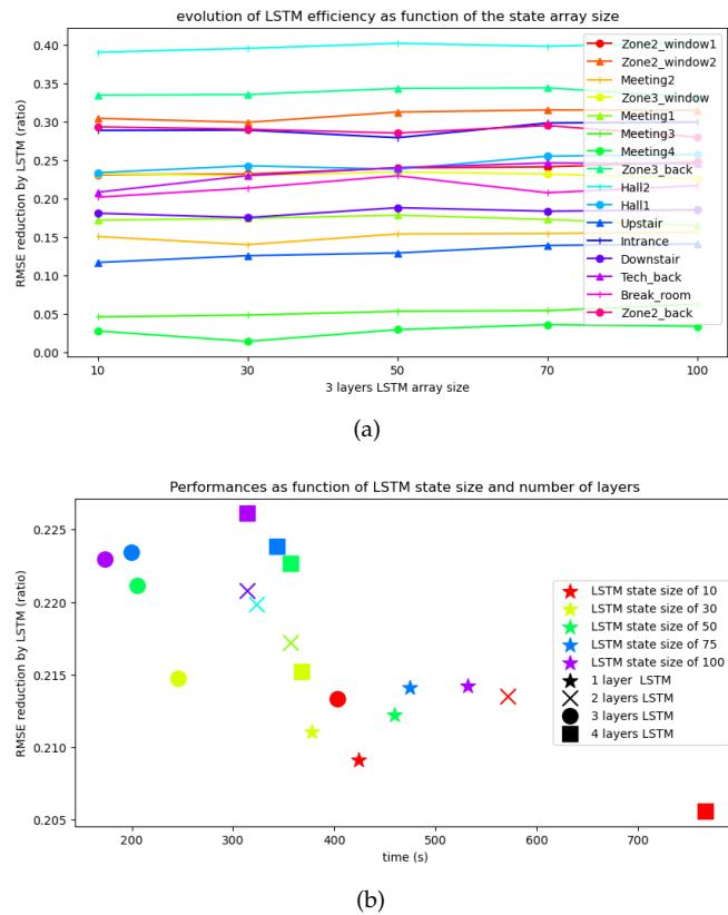
**Figure 3.** Overall performances of LSTM for temperature forecasting on all sensors. (a) Performance as function of architecture used; (b) mean performances and training duration for several LSTM architectures.
