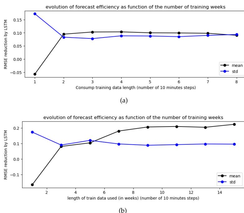
**Figure 7.** Performances of forecasting as a function of training data length. (a) Performances of HVAC consumption forecasting; (b) performances of temperature forecasting.
