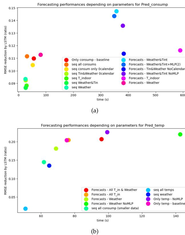
**Figure 4.** Performances as a function of selected forecasting policy and features. (a) HVAC consumption prediction performances; (b) indoor temperature prediction performances.
