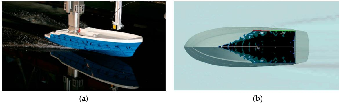
**Figure 9.** Example of dynamic wetted surface and wetted length analysis at  $Fr = 1.96$ . (a) Experimental; (b) numerical. For the numerical data only: wetted keel length (white), wetted chine length (green) and whisker spray length (red).
