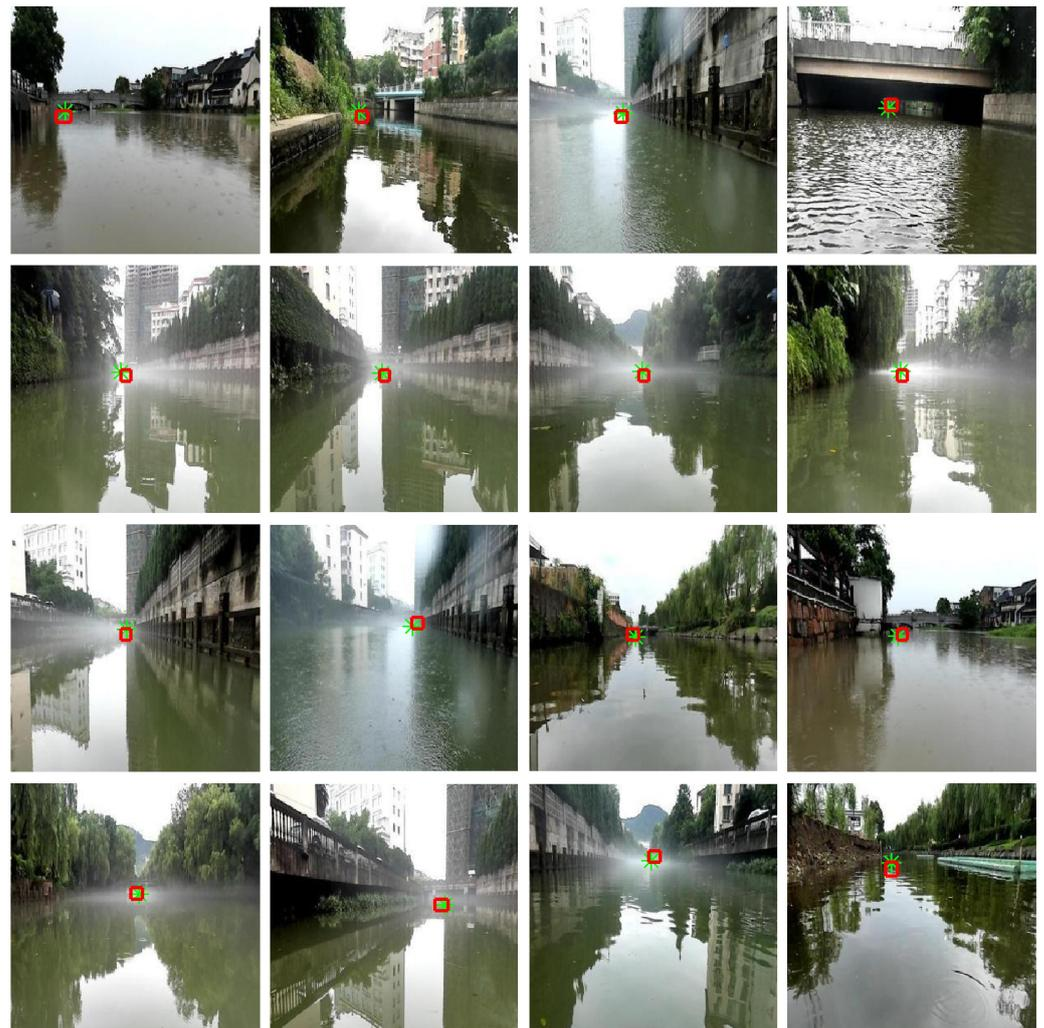
**Figure 7.** Detection of vanishing points in narrow waterway scenarios based on Network R5.
