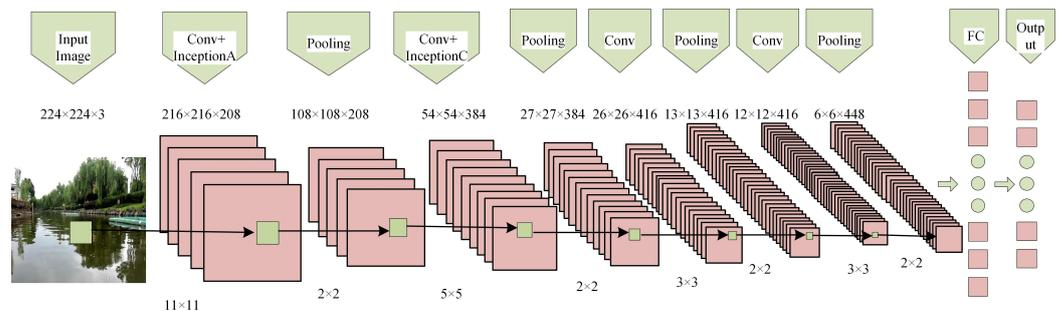
Figure 2. The improved lightweight AlexNet network for vanishing point detection.
