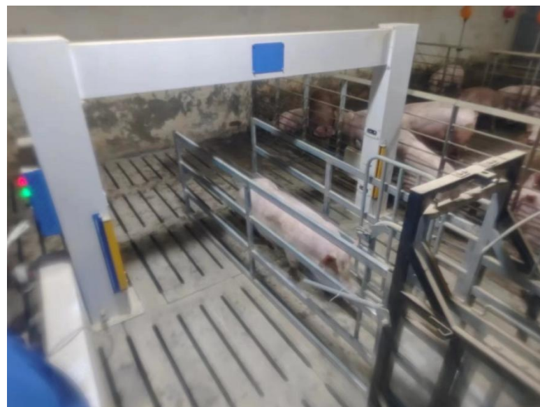
Figure 3. Pig 3D point cloud field acquisition device and acquisition environment.
