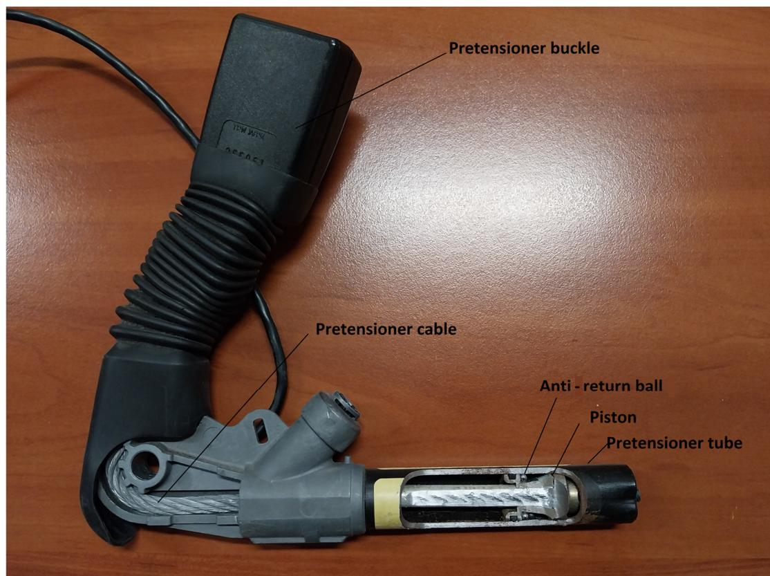
**Figure 1.** The PBP pretensioner, the area of interest for the proposed method.
