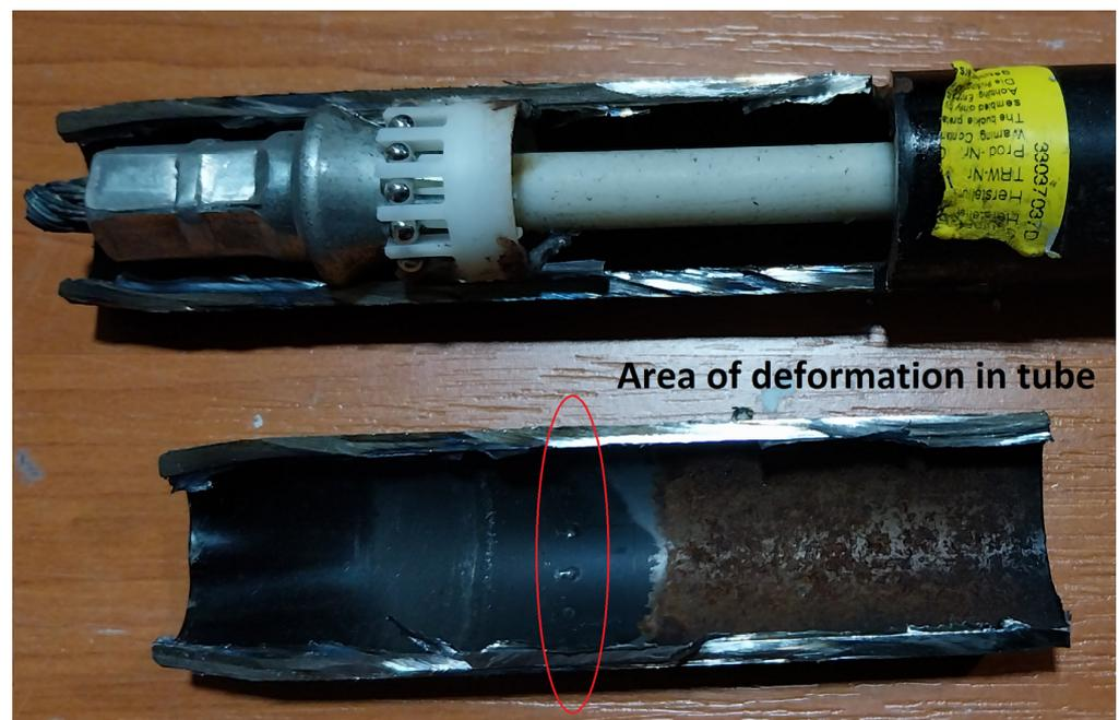
**Figure 5.** Example of cylinder deformed following the functioning of the anti-return pretensioning mechanism PBP.
