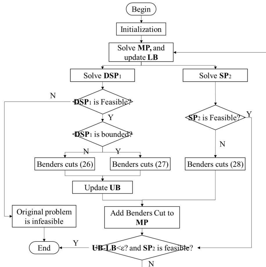
Figure 2. Benders decomposition for MLFLAPs.
