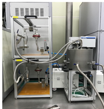
Figure 2. (a) Chassis dynamometer system, (b) gas analyzer, (c) filter sampler for PM and organic marker, and (d) NH 3 analyzer.
