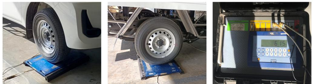
Figure 15. Front wheel weight (left), rear wheel weight (middle), and weight indicator (right).
