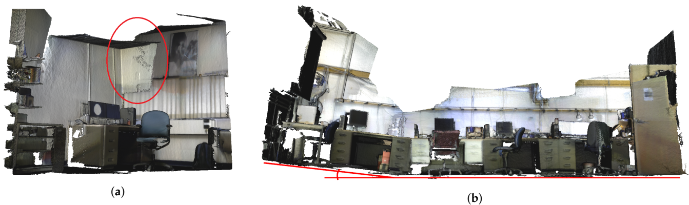
Figure 4. Examples of poor registration in 3D reconstruction from depth frames in the SceneNN dataset [56]. (a) Misalignment of the ceiling in two point clouds, highlighted by the red circle. (b) Deviation from the ground plane and large parts missing from the wall behind the desk. Highlighted by the two red lines and the opening angle, the left part of the room tilts, and the floor is not level.
