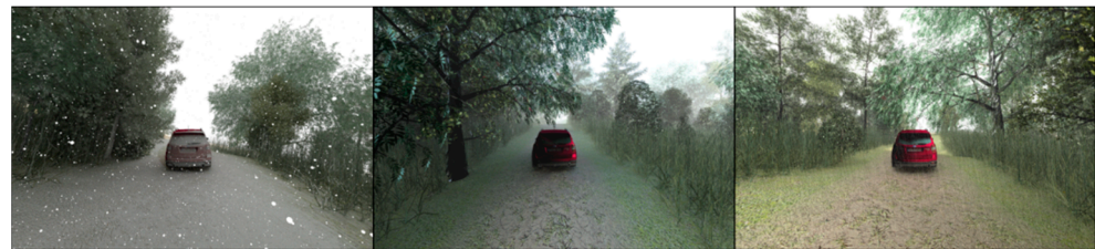
Figure 2. Simulation of snow (left), fog (middle), and rain (right) in MAVS. The terrain was created automatically with MAVS.
