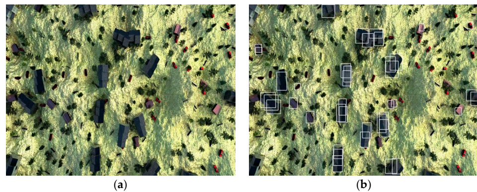
Figure 10. (a) Simulated UAV original image. (b) Detection of “buildings” using RetinaNet, marked in white boxes.
