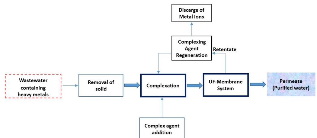
**Figure 1.** Scheme of the complexation-UF hybrid process, adapted from [33].
