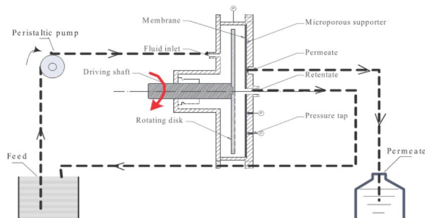
Figure 2. Scheme of the rotating disk enhancing Complex-ultrafiltration process. Adapted with permission from ref. [52]. Copyright 2021 Elsevier.
