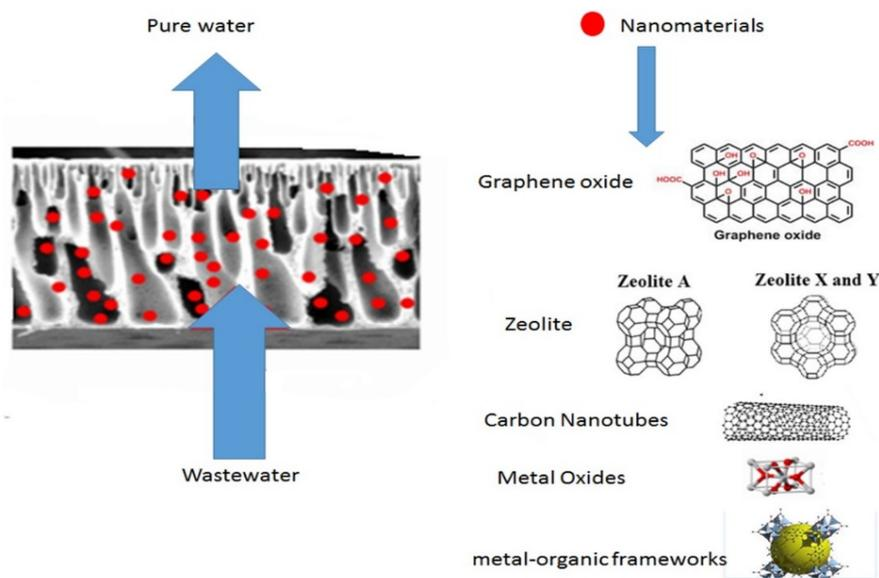
**Figure 3.** Nanomaterial used for nanocomposite membrane preparation. Adapted with permission from ref. [94]. Copyright 2021 Elsevier.
