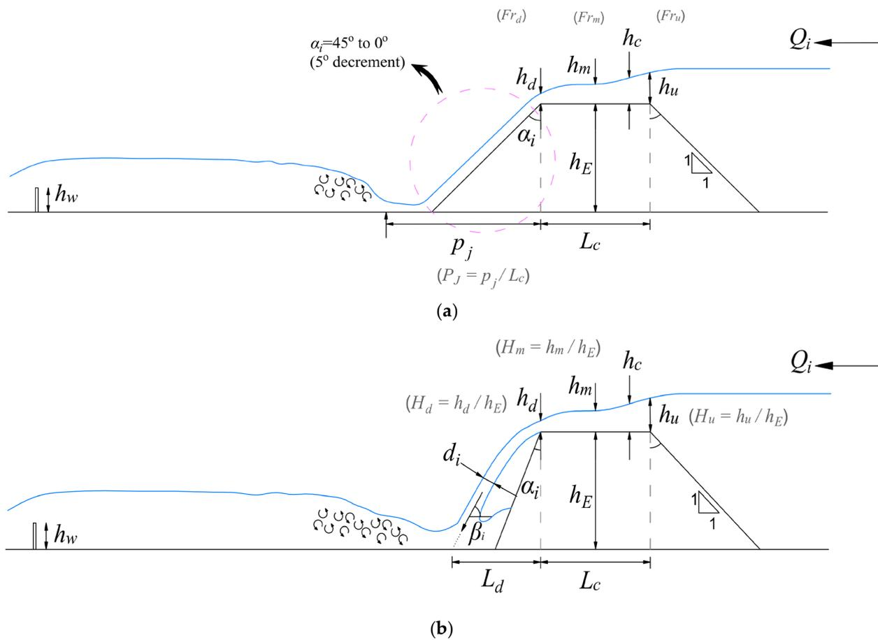
**Figure 3.** Sketch of the experimental setup with nappe flow formation: (a) model setup inside the flume without the vegetation over the crest of EM, (b) schematic of formation of nappe flow without vegetation model over the crest of EM.
