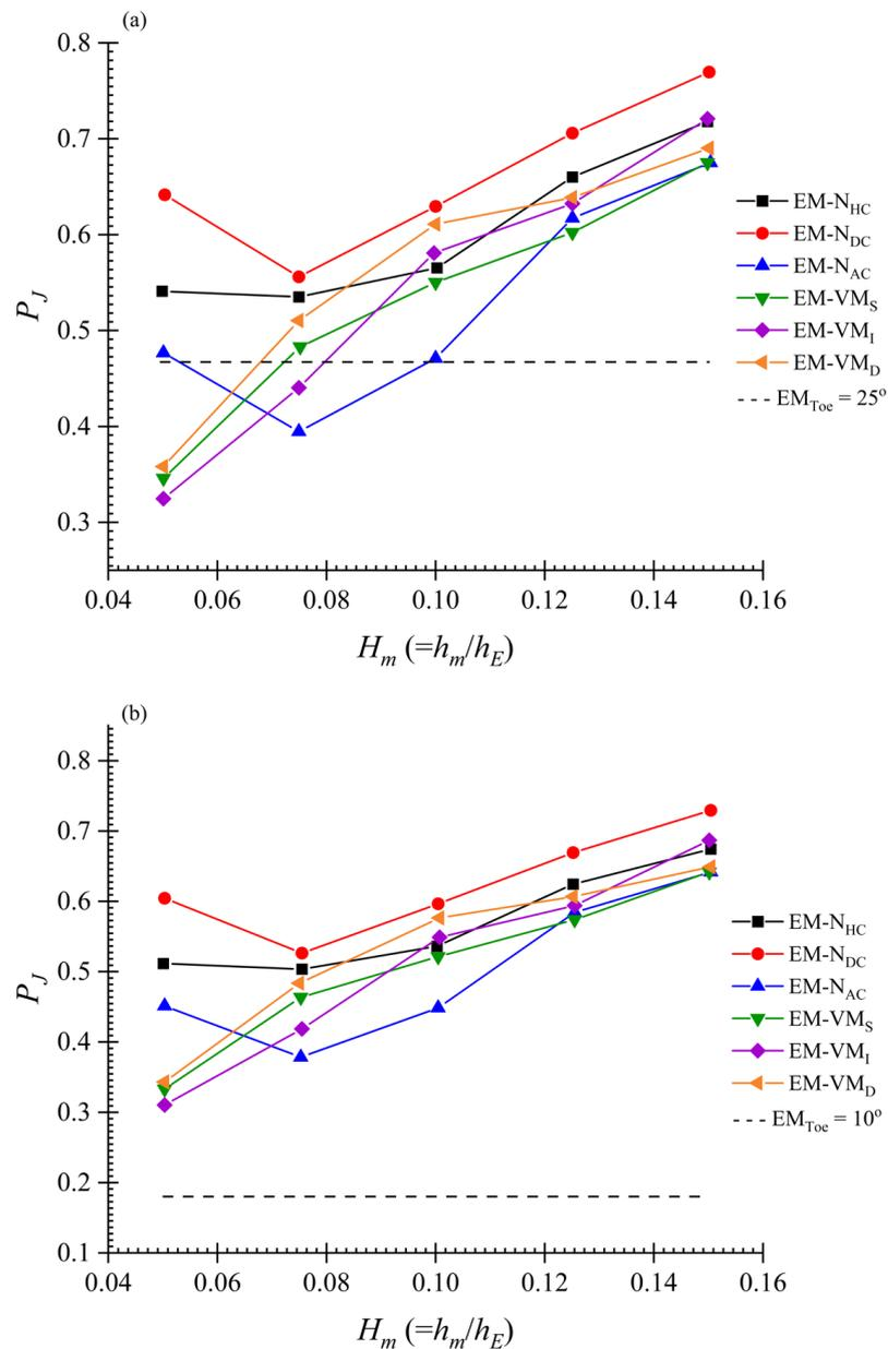
**Figure 10.** Normalized position of the hydraulic jump ( $P_J$ ) with varying normalized overtopping depth ( $H_0$ ): (a)  $25^\circ$  downstream slope; (b)  $10^\circ$  downstream slope.
