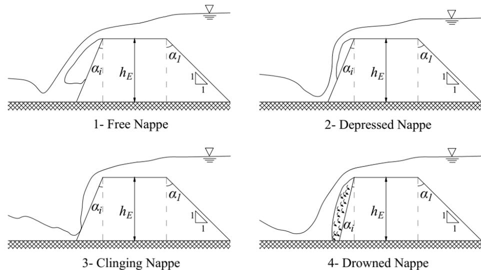
**Figure 4.** Schematic diagram of types of nappe flow.
