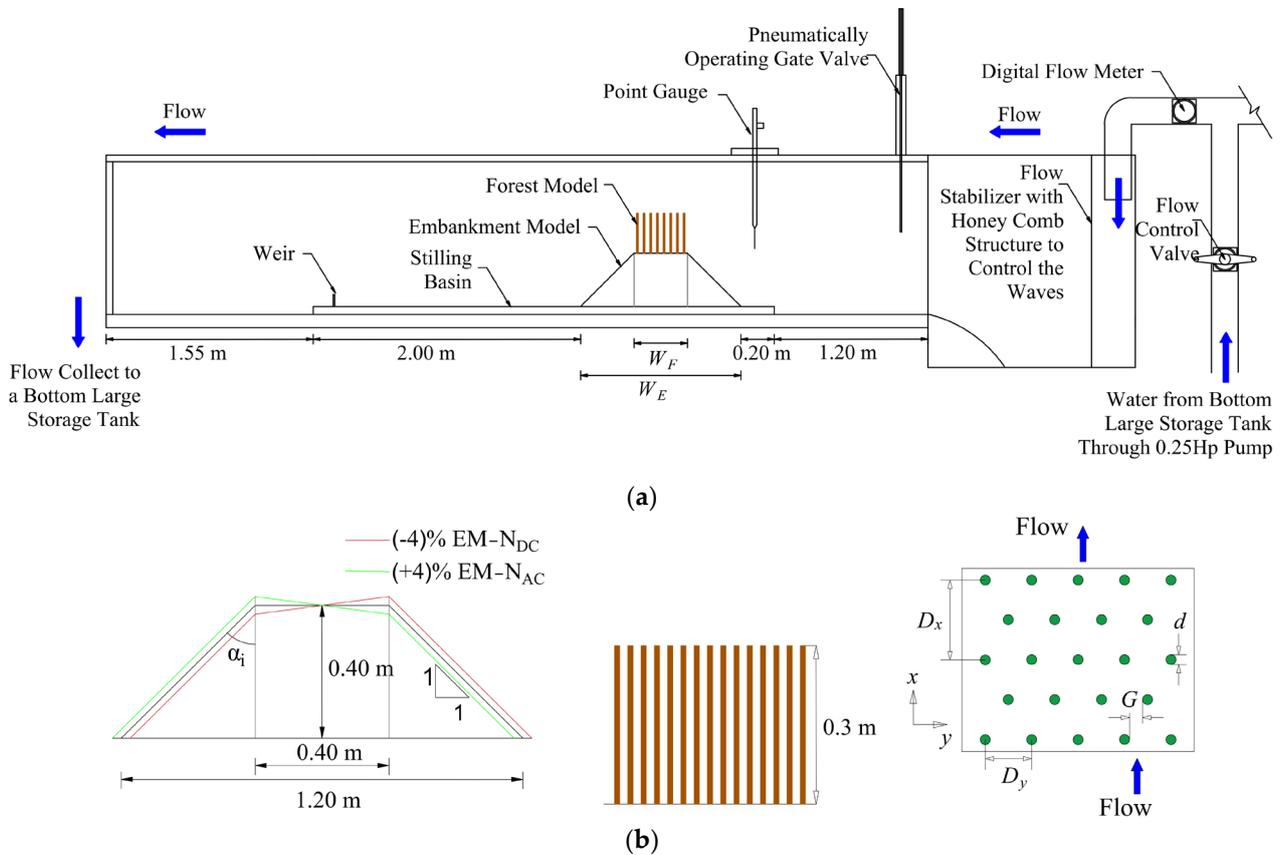
**Figure 2.** Schematic detail of the experimental setup inside the channel: (a) a side view of the experiment flume with embankment (EM) and vegetation model (VM), (b) an embankment model (EM), a side view of the vegetation model (VM), and a plan view of the vegetation model arrangement.
