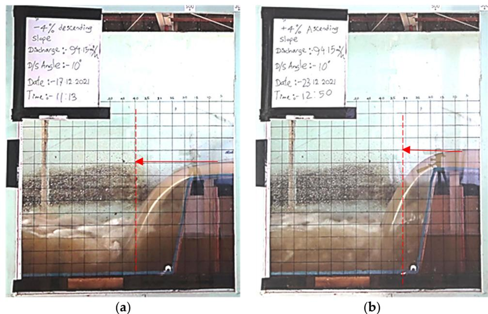
**Figure 9.** Change of the position of the hydraulic jump concerning the type of the nappe flow and downstream slope: (a) −4% descending crest slope (EM-N<sub>DC</sub>) for  $10^\circ$  downstream slope, (b) +4% ascending crest slope (EM-N<sub>AC</sub>) for  $10^\circ$  downstream slope.
