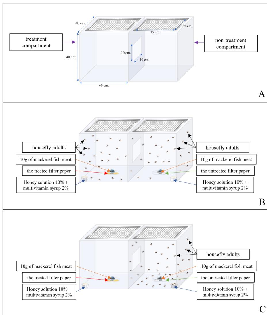
**Figure 1.** Repellent activity bioassay: The test cage was made of five plastic sheets (40 × 40 cm) and one screen sheet (35 × 35 cm) at the top of the cage, and the two compartments were connected by a rectangular hole (10 × 10 cm) in the middle of the cage (A). The first compartment on the left side contained a tested formulation, and the second compartment on the right contained the solvent (B). At the end, repellency could be observed and quantified (C).
