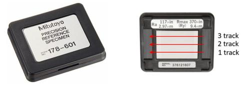
Figure 4. Precision roughness reference specimen with the measuring direction.
