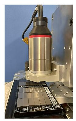
Figure 13. SR-Test Precision during the measurement of roughness standard samples.
