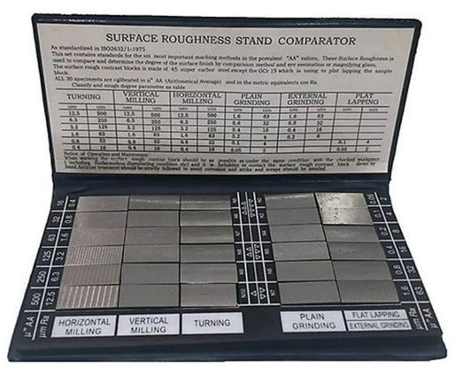
Figure 11. Surface roughness comparator standards composite set.
