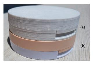
Figure 5. Surface finish comparison of (a) FFF and (b) IM compact.
