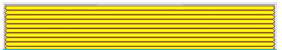
**Figure 14.** A 0.33 mm layer thickness 3D-printed specimen.
