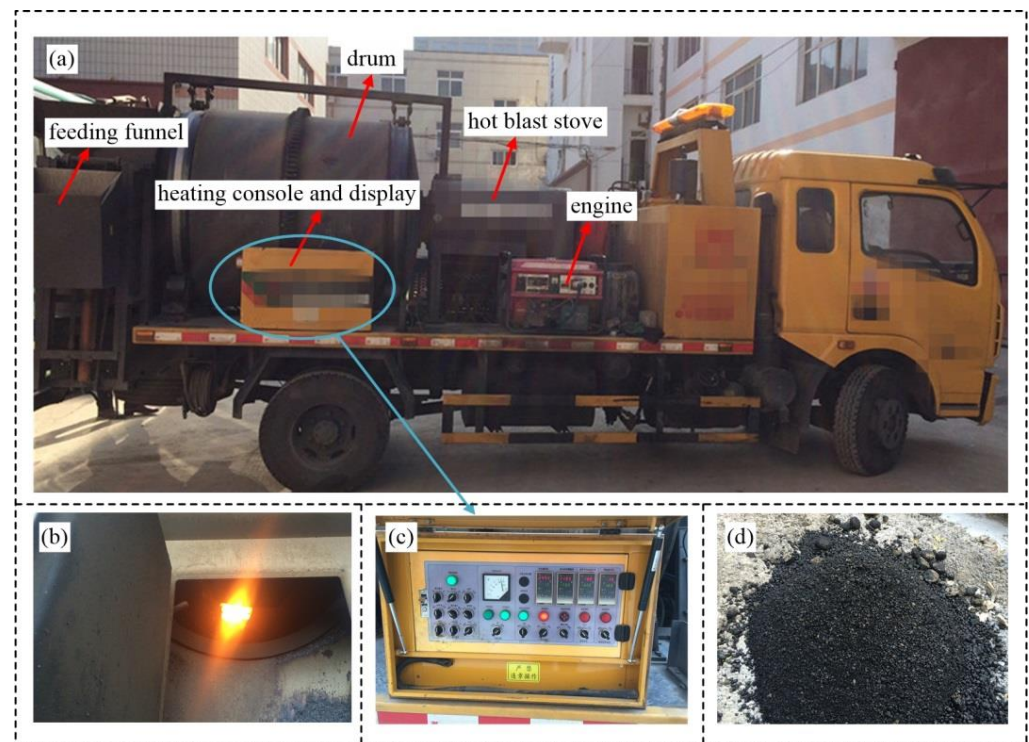
Figure 3. Heating test of bituminous mixture: (a) experimental equipment for heating the bituminous mixture; (b) bituminous mixture being heated in the drum; (c) heating console and temperature meter of bituminous mixture; (d) bituminous mixture after heating.
