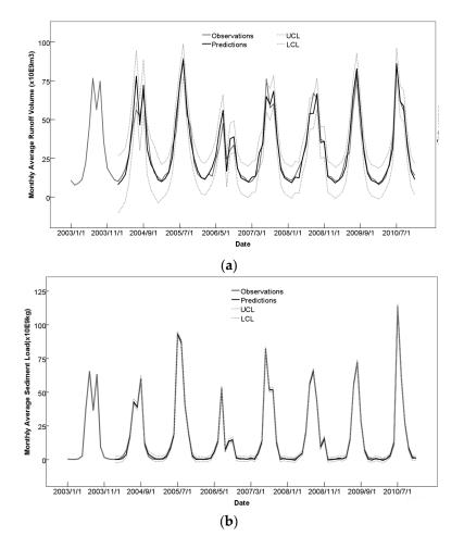
Figure 9. Predictions by ARIMA model: (a) Runoff; (b) Sediment.
