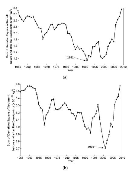
**Figure 5.** Fisher's ordered clustering curves of runoff and sediment into the TGP: (**a**) Runoff; (**b**) Sediment.
