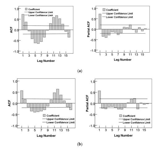
Figure 7. ACF and PACF of Runoff and Sediment into the TGP: (a) Runoff; (b) Sediment.
