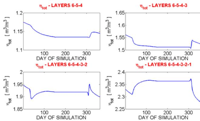
**Figure 12.**  $\eta_i$  (volumetric ice content) trends relative to the sensitivity test summarized in Figure 9, for the fourth layer (top left), the third layer (top right), second layer (bottom left) and first layer (bottom right).
