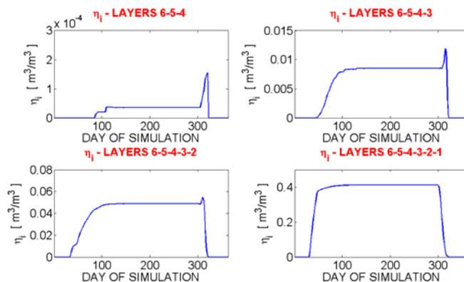
At the beginning of each time step, the quantity  $\eta_{i,tot}$ , *i.e.*, the total volumetric ice content in all soil layers, is calculated. If  $\eta_{i,tot}$  is greater than the minimum value  $0.01 \text{ m}^3/\text{m}^3$  (*i.e.*, if there is a significant quantity of ice in soil), the variable  $\eta_{tot,correct}$  is computed by setting to zero the hydraulic diffusivity ( $D_{w\eta} = 0$ ), in order to neglect the water fluxes among the soil layers due to the humidity gradient. In this
