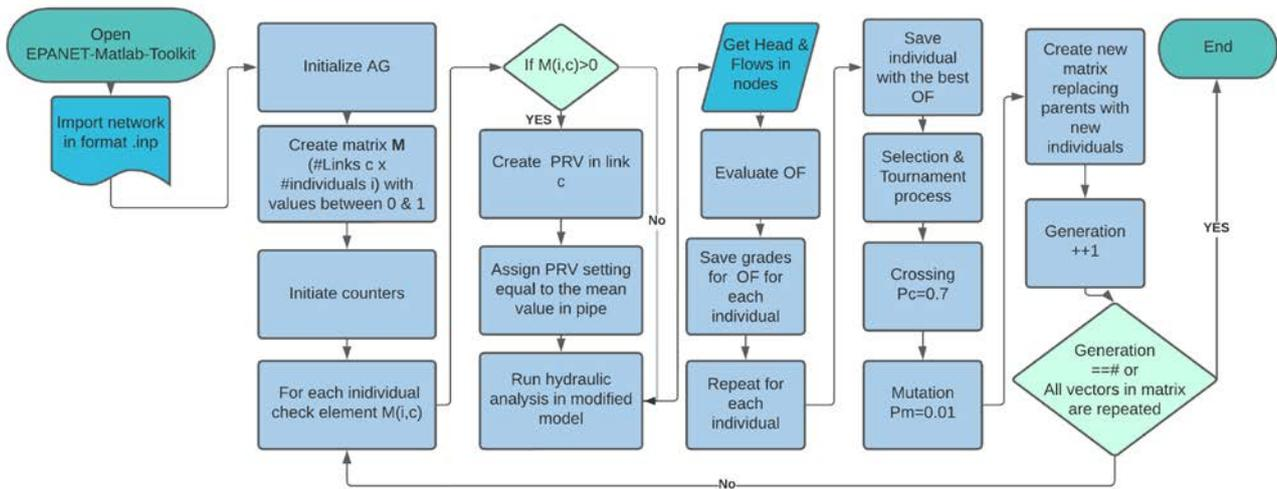
**Figure 3.** RCGA process for diminishing Head & Pressure. Where # is number and ++ means plus one, and == means conditional if equal to.
