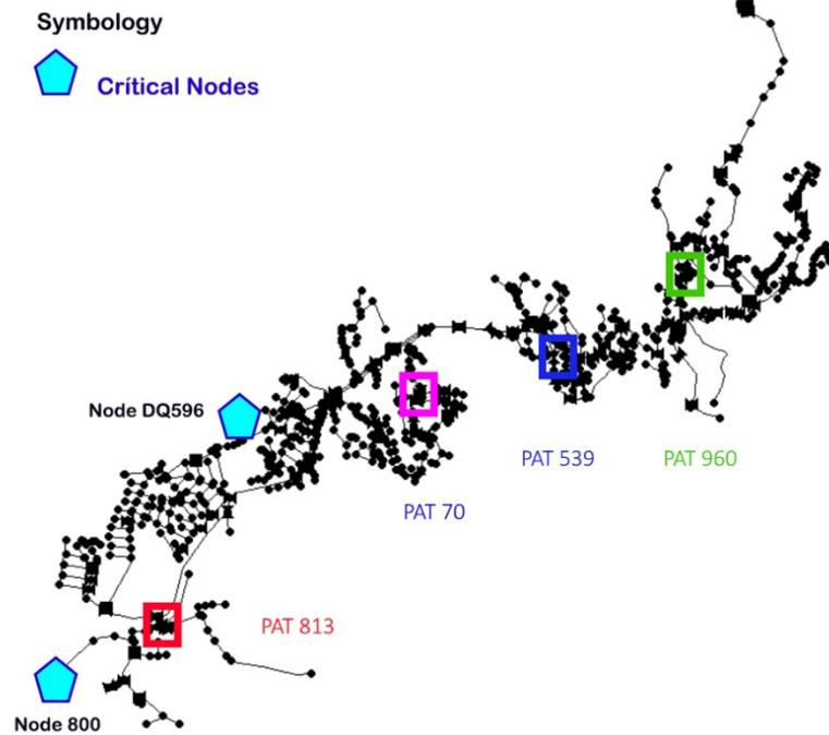
Figure 8. PAT location and critical nodes obtained by the methodology described.
