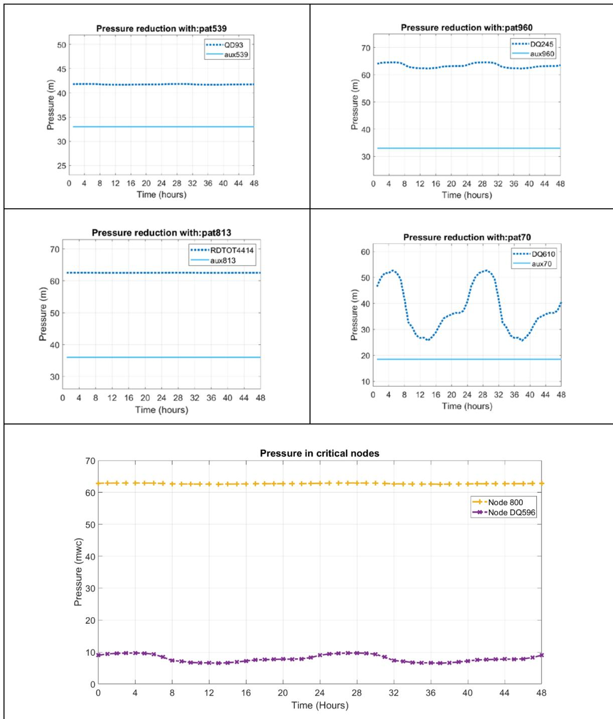
**Figure 9.** Pressures for PATs and critical nodes in sector 8–12 on extended period.
