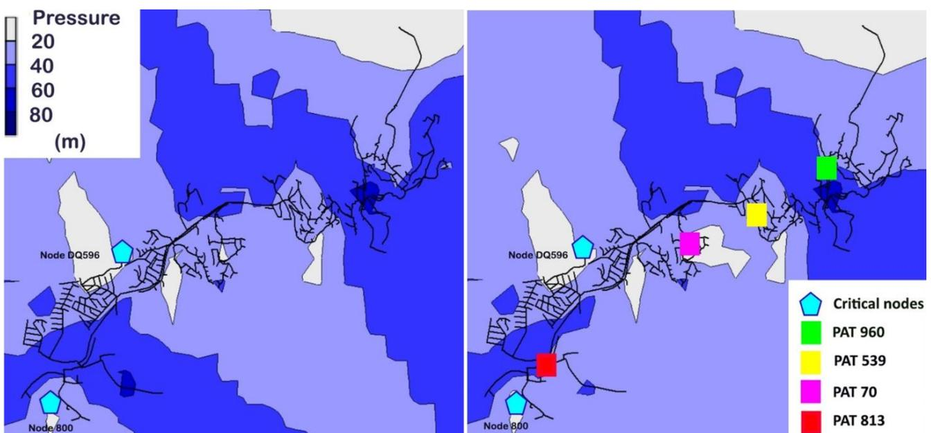
**Figure 12.** Pressure contour map for network 8–12 statistics maximum from EPANET. Initial network (left contour) and network with PATs (right contour).
