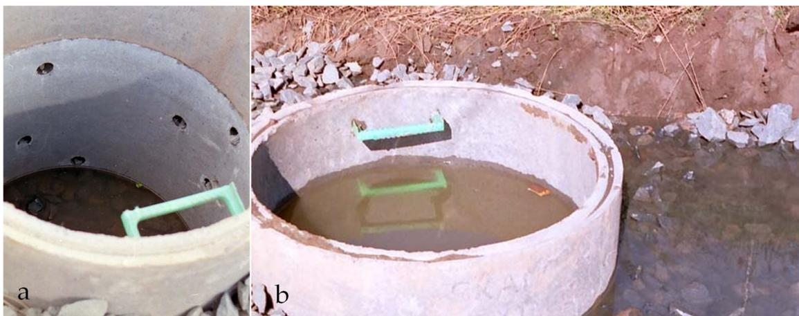
**Figure A24.** Abstraction device (1.2 m OD), which was designed to access water within a shallow groundwater mound. (a), constructed device showing a perforated chamber surrounded by coarse gravel, with interception of the feather edge of the groundwater mound at its base. The water level is >1.2 m below the ground surface; (b), the same abstraction infiltration device 24 h later, showing the groundwater mound surface located 0.2 m below the ground surface.
