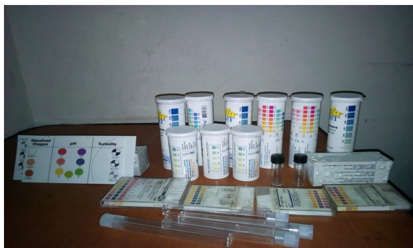
Figure 5. LaMotte© tests used to measure field water quality parameter by citizen scientists.
