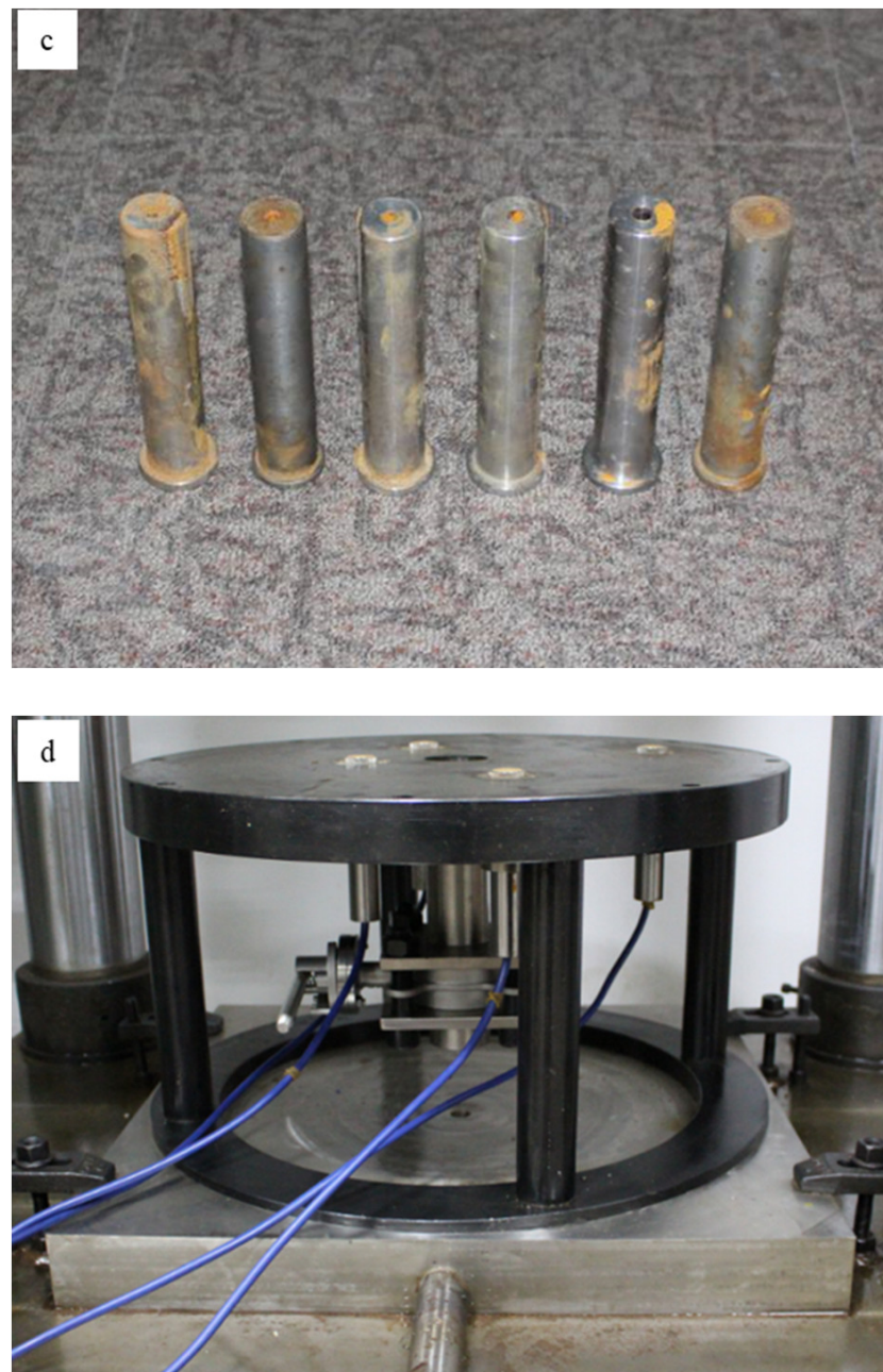
Figure 4. Base of the testing chamber: (a) picture of the testing chamber; (b) structural plan of the testing chamber; (c) karst conduits of different sizes; (d) instantaneous opening device for the karst conduit.
