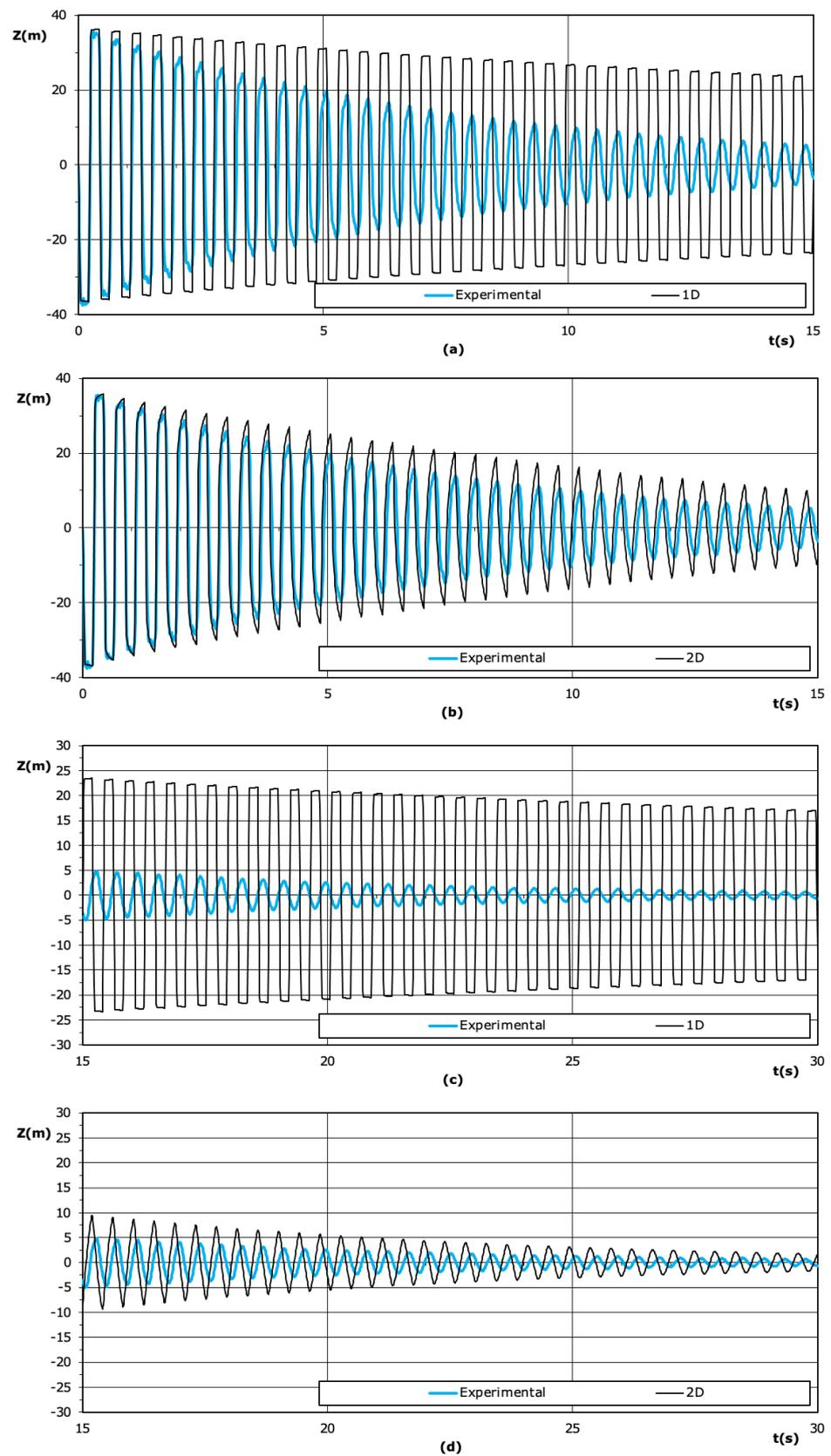
**Figure 5.** Comparison of head oscillations computed with the 1D or 2D model without free gas with the experimental results for Test L3: (a) 1D model,  $t = 0 - 15$  s; (b) 2D model,  $t = 0 - 15$  s; (c) 1D model,  $t = 15 - 30$  s; (d) 2D model,  $t = 15 - 30$  s.
