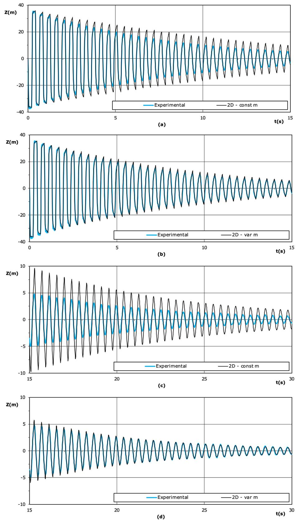
**Figure 6.** Comparison of head oscillations computed with the 2D model with constant or variable mass of free gas with the experimental results for Test L3: (a) 2D model with constant mass of free gas,  $t = 0 - 15$  s; (b) 2D model with variable mass of free gas,  $t = 0 - 15$  s; (c) 2D model with constant mass of free gas,  $t = 15 - 30$  s; (d) 2D model with variable mass of free gas,  $t = 15 - 30$  s.
