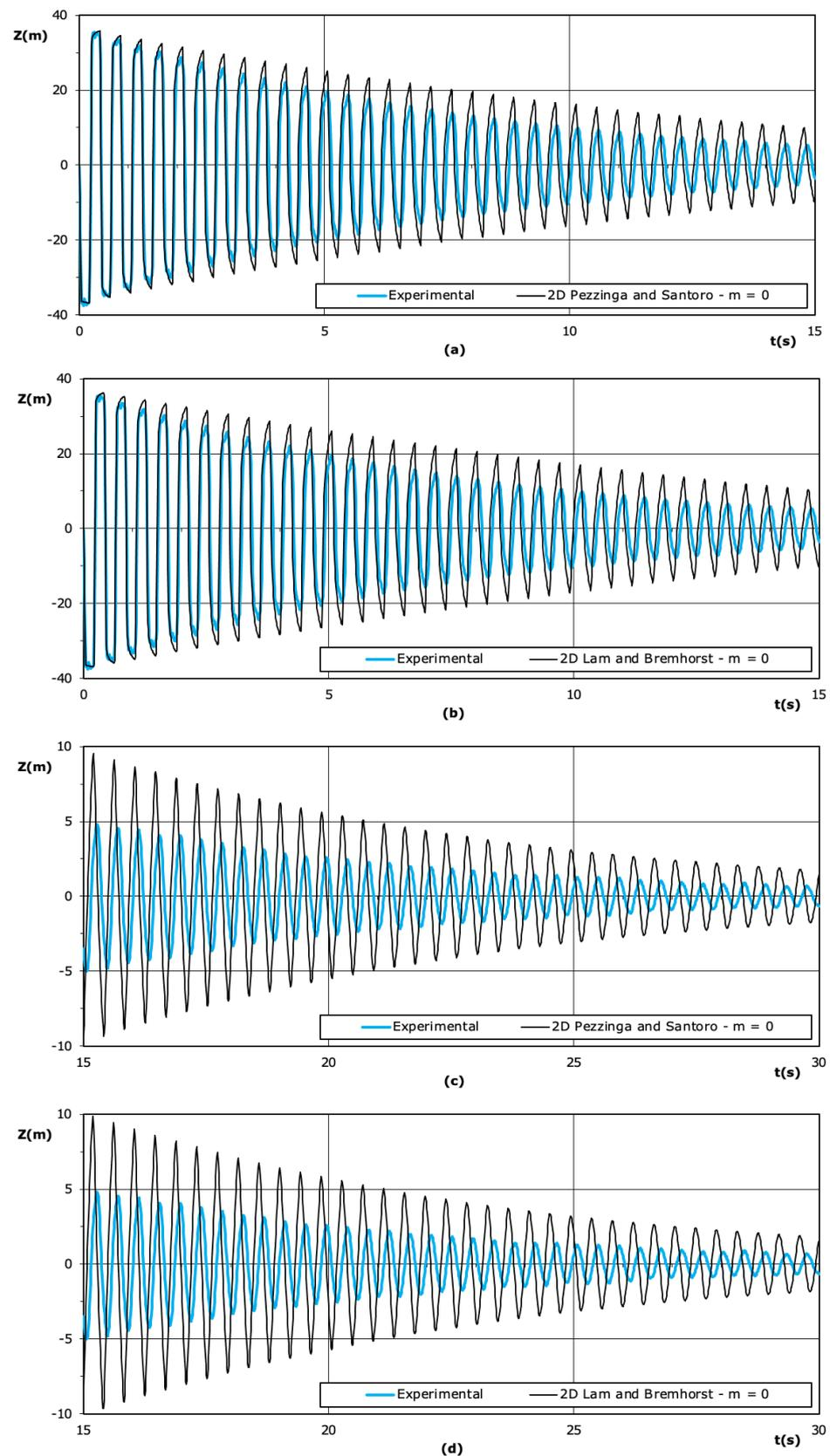
**Figure 7.** Comparison of head oscillations computed with the 2D present model or with the Lam and Bremhorst [23] model without free gas with the experimental results for Test L3: (a) 2D present model,  $t = 0 - 15$  s; (b) 2D Lam and Bremhorst model,  $t = 0 - 15$  s; (c) 2D present model,  $t = 15 - 30$  s; (d) 2D Lam and Bremhorst model,  $t = 15 - 30$  s.
