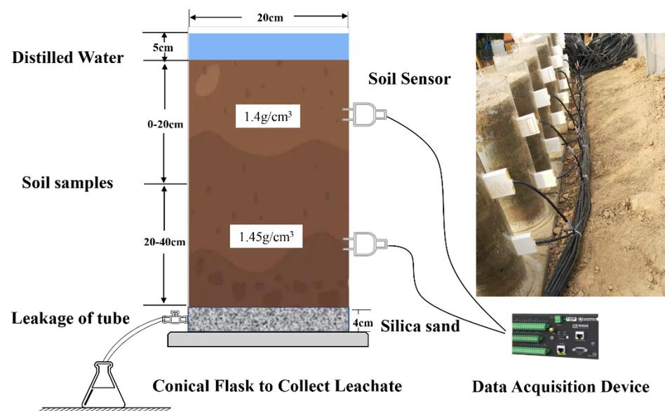
Figure 1. Design diagram of soil column experiment.
