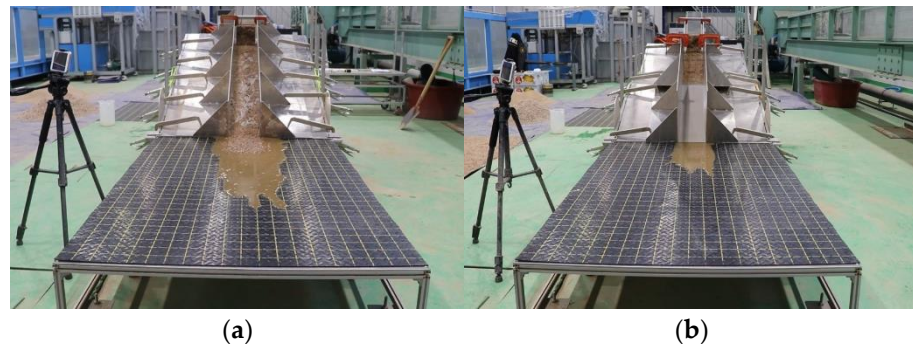
Figure 5. Examples of laboratory tests: (a) Example of a straight channel test ( \alpha = 20^\circ and C_V = 0.50 ); and (b) example of a single-berm channel test ( \alpha = 20^\circ and C_V = 0.50 ).
