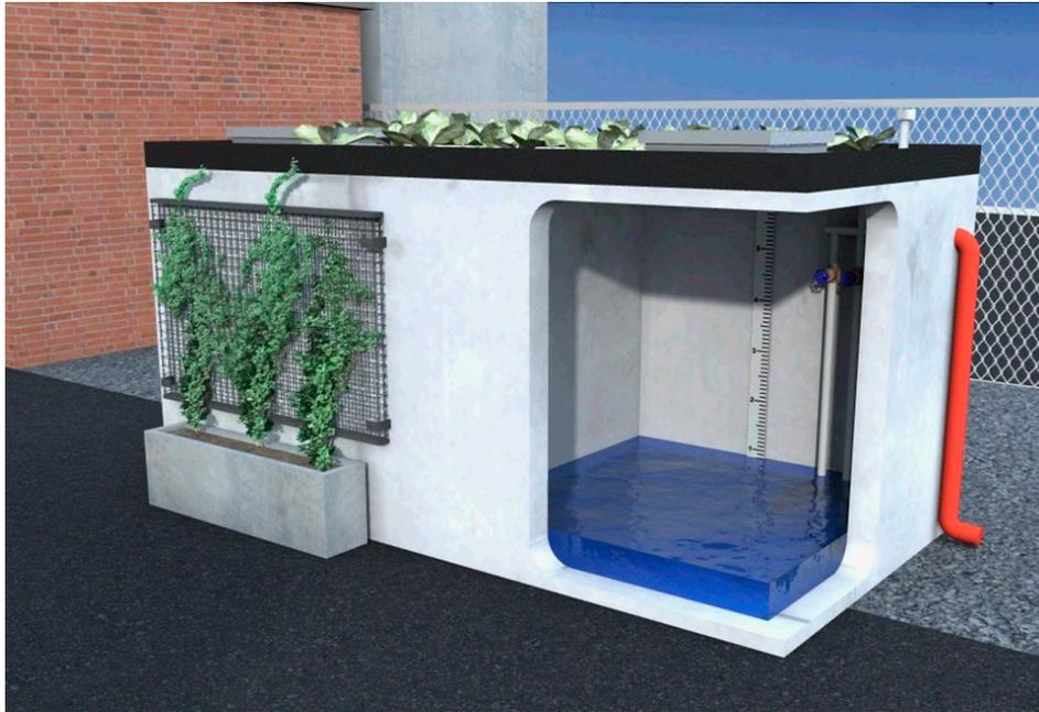
Figure 2. Cistern rendering showing concrete green tank structure with vegetated roof, planter with green screen and overflow pipe.
