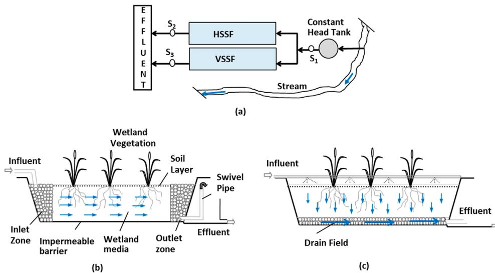
Figure 3. (a) Wetland arrangement: S<sub>1</sub>, S<sub>2</sub> and S<sub>3</sub> are sampling points. (b) Schematic diagram of a horizontal subsurface flow (HSSF) wetland system. (c) Schematic diagram of a vertical subsurface flow (VSSF) wetland system.
