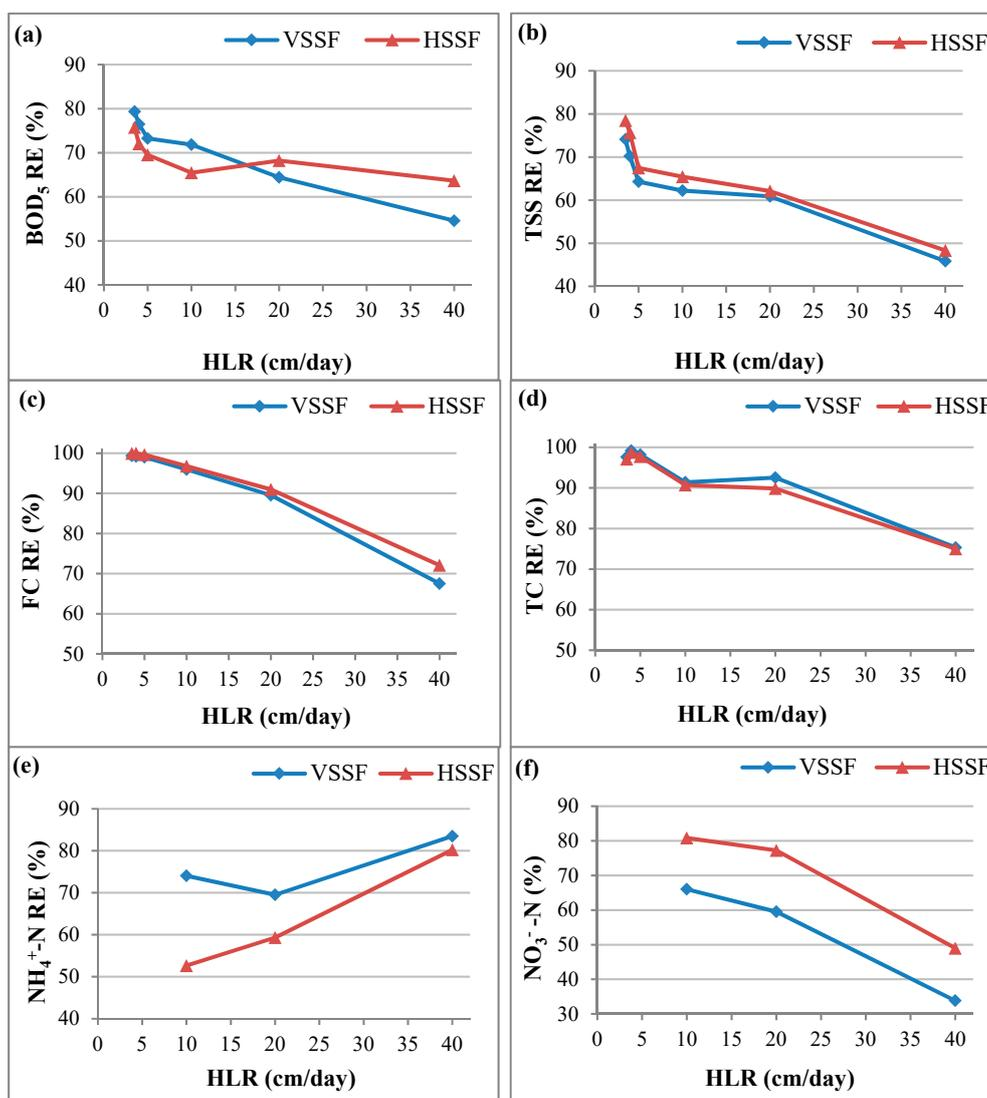
**Figure 7.** Variation of removal efficiencies (RE) of (a) BOD<sub>5</sub>, (b) TSS, (c) FC, (d) TC, (e) NH<sub>4</sub><sup>+</sup>-N, and (f) NO<sub>3</sub><sup>-</sup>-N in VSSF and HSSF wetland units versus HLR.
