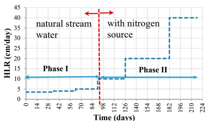
**Figure 5.** Sequence of water application in VSSF and HSSF wetland units. HLR: hydraulic loading rate.
