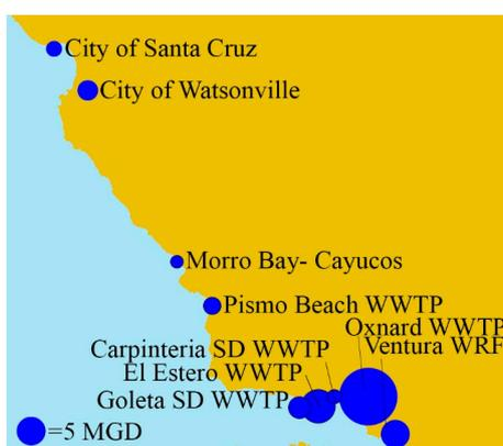
**Figure 6.** Location and average dry weather effluent flow rate rates of WWTFs in the Central Coast region that discharge at least 3.8 MLD (1 MGD). WRF, Water Reclamation Facility.
