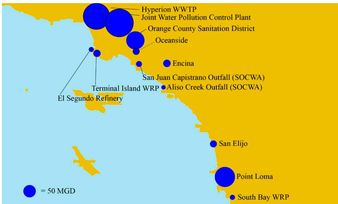
**Figure 7.** Location and average dry weather effluent flow rates of WWTFs in the South Coast region that discharge at least 3.8 MLD (1 MGD).
