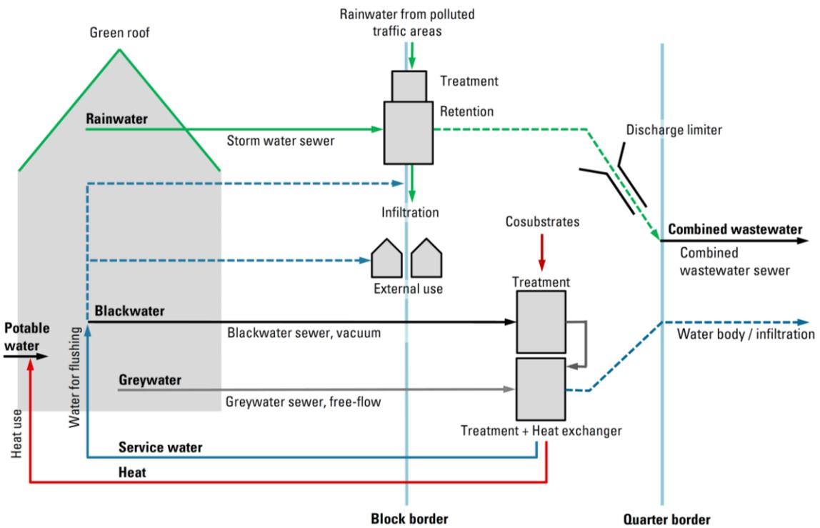
Figure 3. Scheme of the Hamburg Water Cycle (with heat recovery) technical option at the quarter level (based on [31]).
