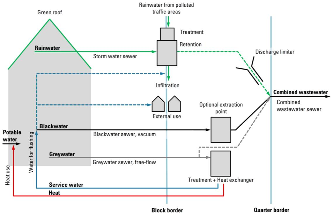
Figure 2. Scheme of the ConvGrey Hamburg technical option at the quarter level (based on [31]).
