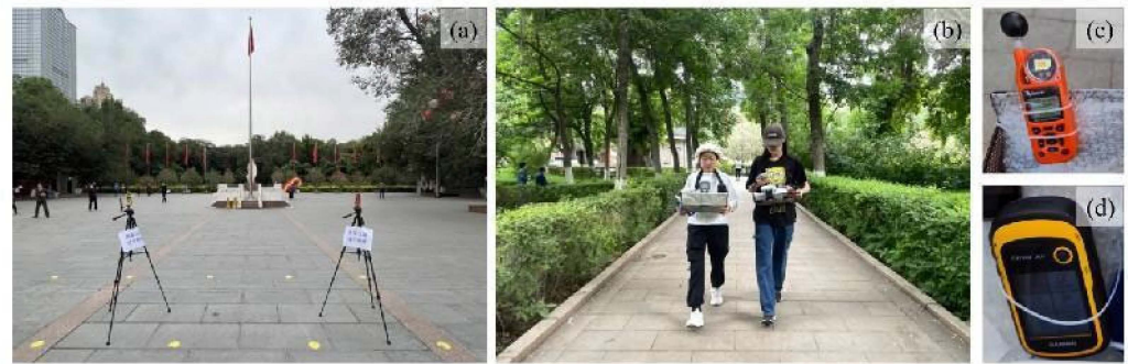
Figure 2. Field monitoring: (a) fixed-point measuring instrument; (b) mobile monitoring personnel and instruments; (c) Kestrel 5400 mobile monitoring instrument; (d) Garmin eTrex 201 mobile monitoring instrument.
