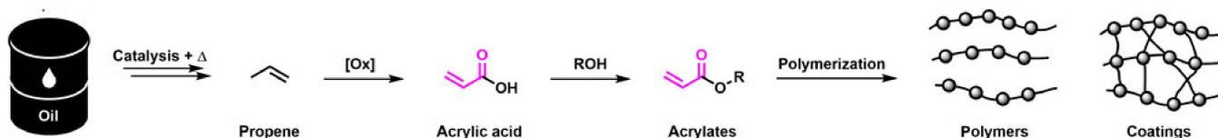
**Figure 11.** Traditional petrochemical-based synthetic approach to polyacrylates.
