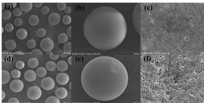
**Figure S1.** SEM of the surface of epoxy resin Lx-105s before (a, b, c) and after (d, e, f) immobilization of Est<sub>BAS</sub>ΔSP. Magnification: a, d  $\times 100$ ; b, e  $\times 500$ ; c, f  $\times 15$  k.
