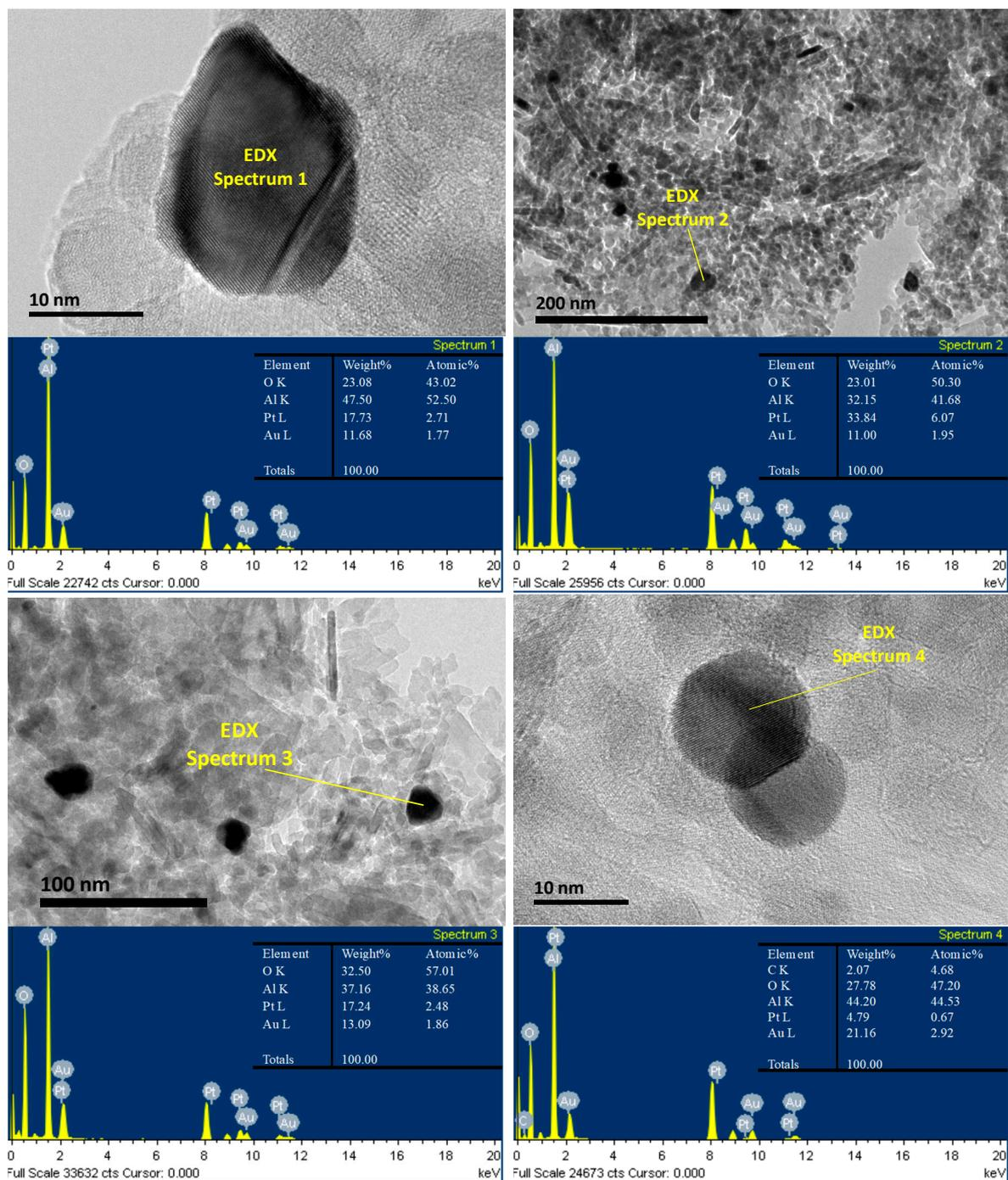
**Figure S3.** HR-TEM images of Pt-Au/Al catalyst showing examples of particles with their corresponding EDX data.
