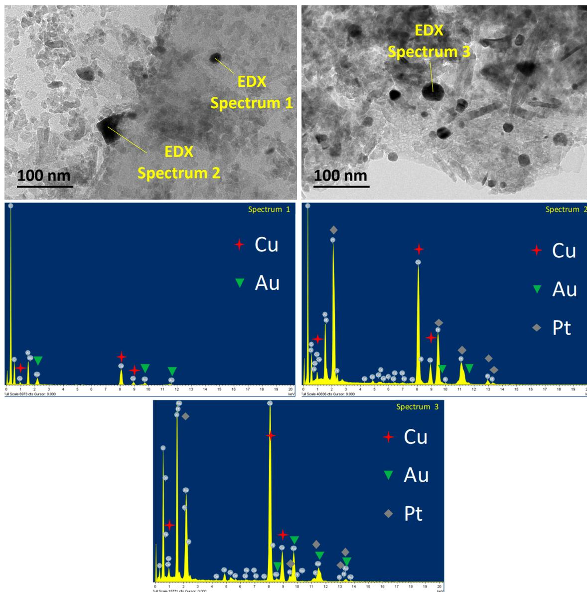
**Figure S8.** HR-TEM images of Pt-Au/Ce-Al catalyst showing examples of particles with their corresponding EDX data.
