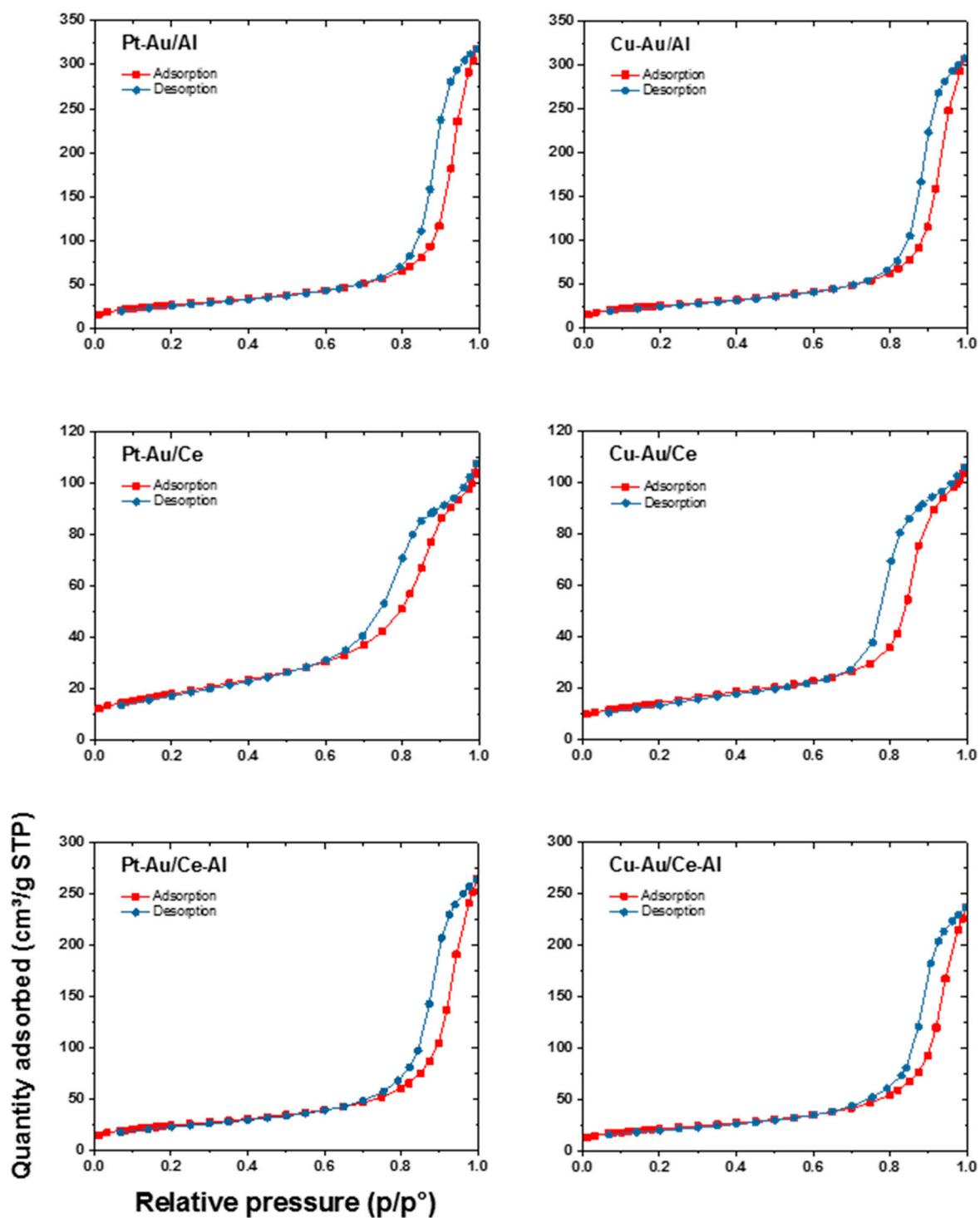
Figure S1.  $N_2$  adsorption isotherms of the prepared bimetallic catalysts.
