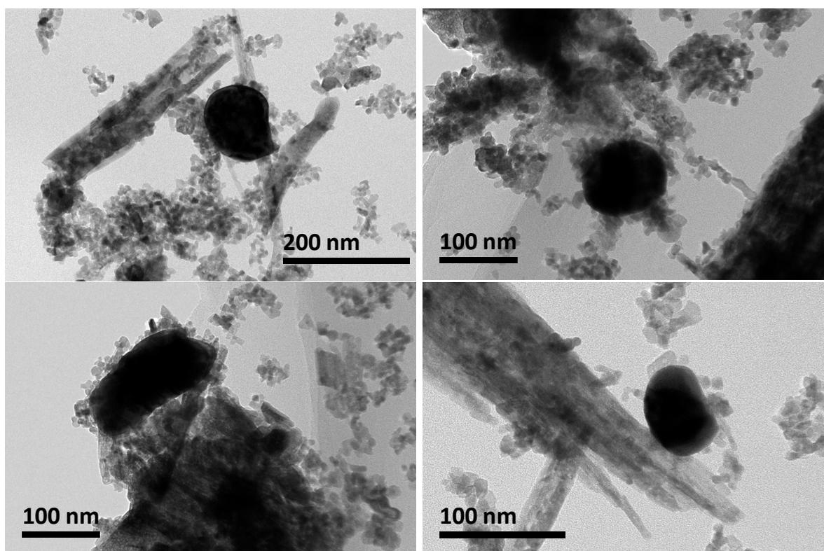
Figure S5. HR-TEM images of Pt-Au/Ce catalyst showing examples of particles.
