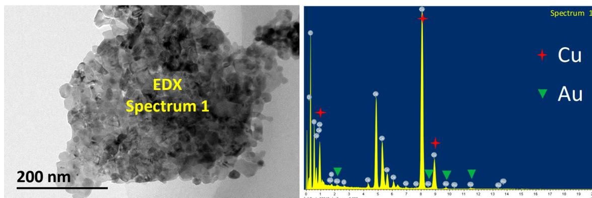
Figure S6. HR-TEM image of Cu-Au/Ce catalyst with corresponding EDX data.
