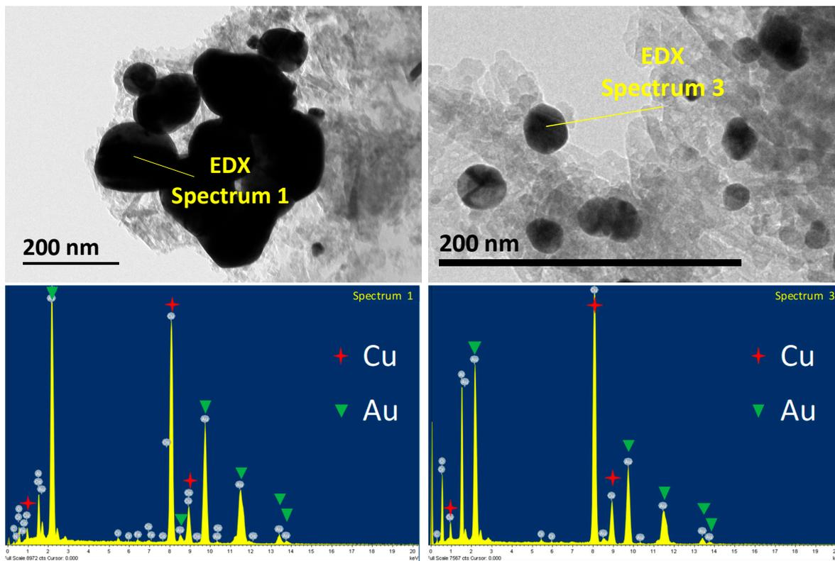
Figure S4. HR-TEM images of Cu-Au/Al catalyst showing examples of particles with their corresponding EDX data.
