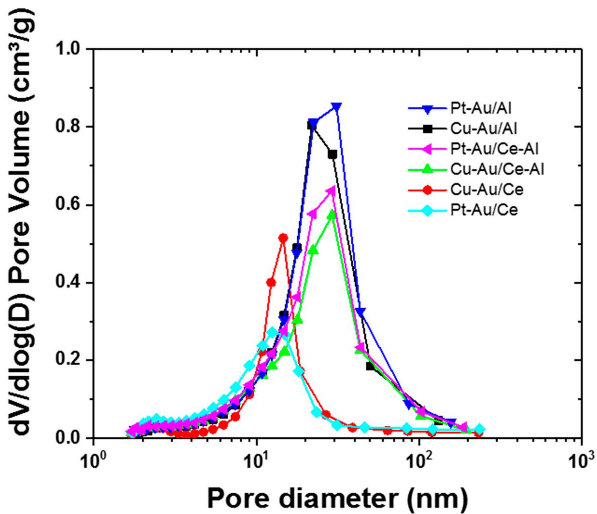
Figure S2. Pore size distributions of the prepared bimetallic catalysts.
