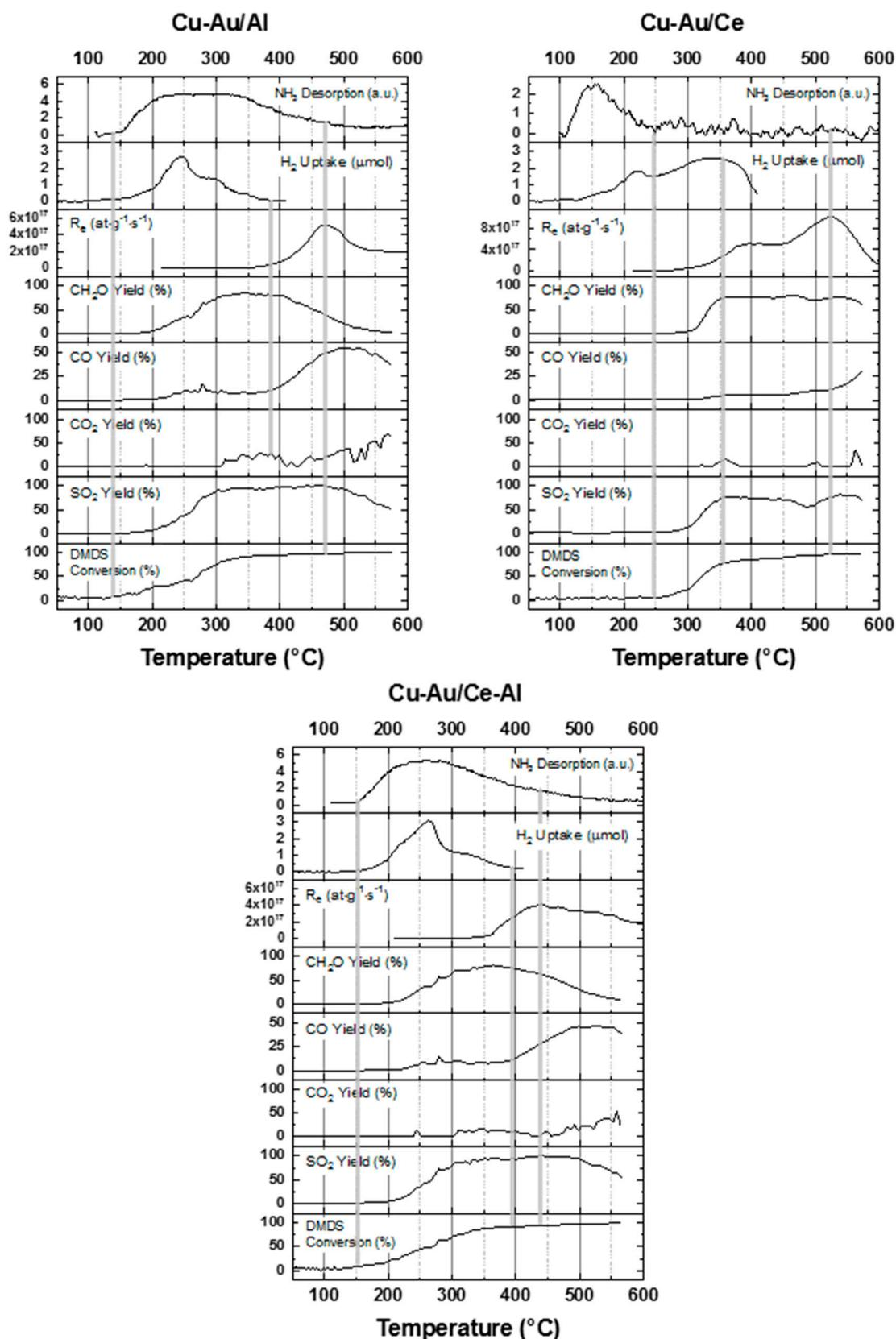
**Figure S11.** DMDS conversion, product yields (SO<sub>2</sub>, CO<sub>2</sub>, CO, and CH<sub>2</sub>O), oxygen exchange rate, H<sub>2</sub> uptake, and NH<sub>3</sub> desorption results for the Cu-Au/Al, Cu-Au/Ce, and Cu-Au/Ce-Al catalysts.
