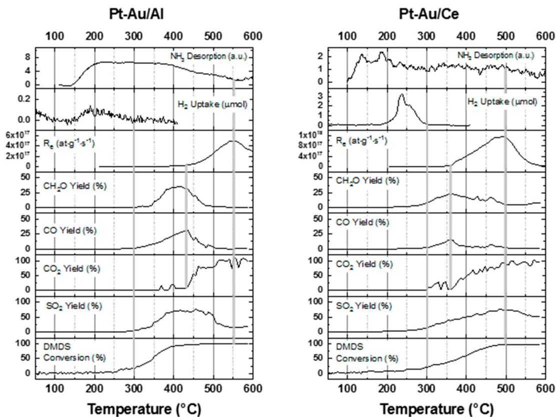
Figure S10. DMDS conversion, product yields ( $\text{SO}_2$ ,  $\text{CO}_2$ ,  $\text{CO}$ , and  $\text{CH}_2\text{O}$ ), oxygen exchange rate,  $\text{H}_2$  uptake, and  $\text{NH}_3$  desorption results for the Pt-Au/Al and Pt-Au/Ce catalysts (Figure 15 shows corresponding graph for the Pt-Au/Ce-Al catalyst).
