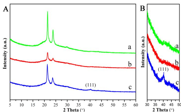
**Figure 5.** X-ray diffraction spectroscopy (XRD) pattern (A) with zoom-in region (B) of PEI/PCL fibers with the weight ratios of 10:90 (a) and 35:65 (b) and PEI/PCL@PdNPs composite (c).
