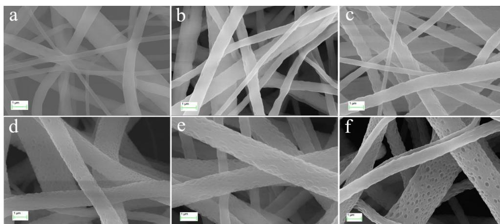
**Figure 2.** SEM images of AuNPs coated PEI/PCL electrospun fibers with different weight ratios ((w/w) (a), 10:90; (b), 15:85; (c), 20:80; (d), 25:75; (e), 30:70; (f), 35:65).
