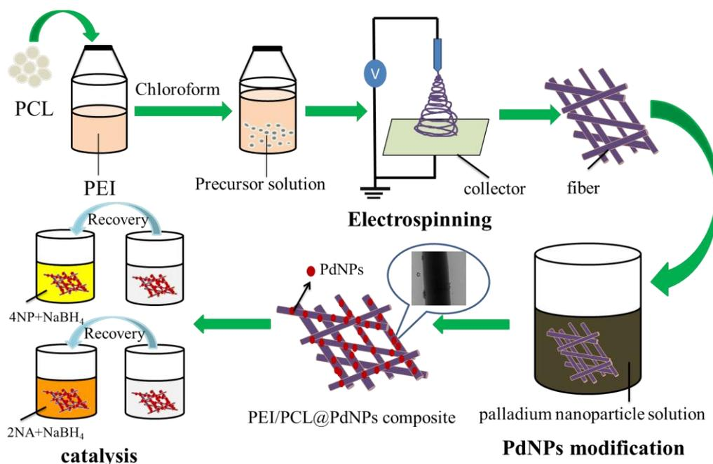
**Figure 1.** Preparation process of polyethyleneimine/polycaprolactone/Pd nanoparticles (PEI/PCL@PdNPs) composite and its catalytic performance.
