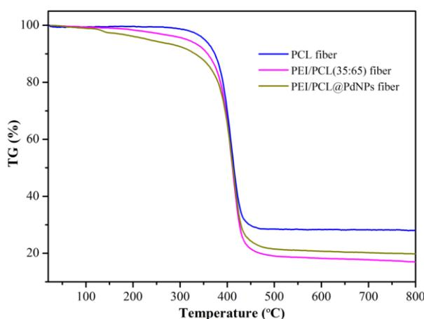
**Figure 6.** Thermogravimetry (TG) curves of the prepared PCL fibers and PEI/PCL fibers with the weight ratios of 35:65 and PEI/PCL@PdNPs composite.
