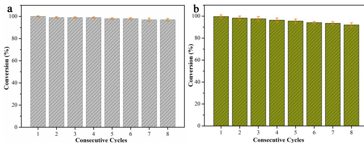
**Figure 9.** Recyclability test of PEI/PCL@PdNPs catalyst for the reduction of 4-NP (a) and 2-NA (b).
