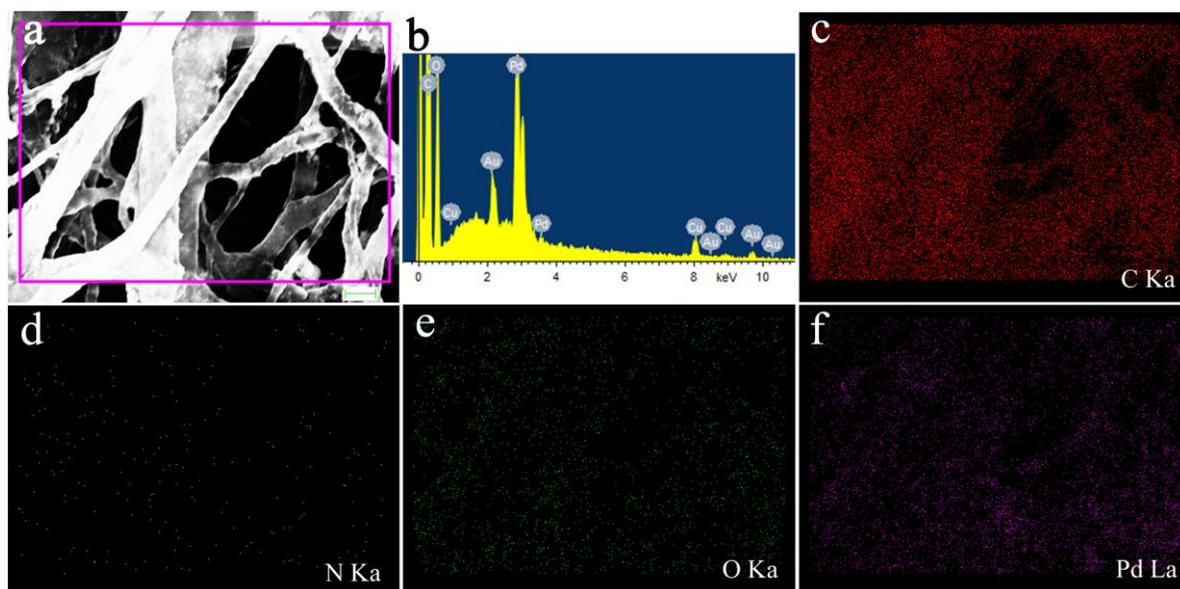
**Figure 4.** Scanning electron microscope (SEM) and EDS images of as-prepared PEI/PCL@PdNPs composite (a,b) and C/O/N/Pd elemental mapping (c–f). The scale bar in image a represent 1  $\mu\text{m}$ .
