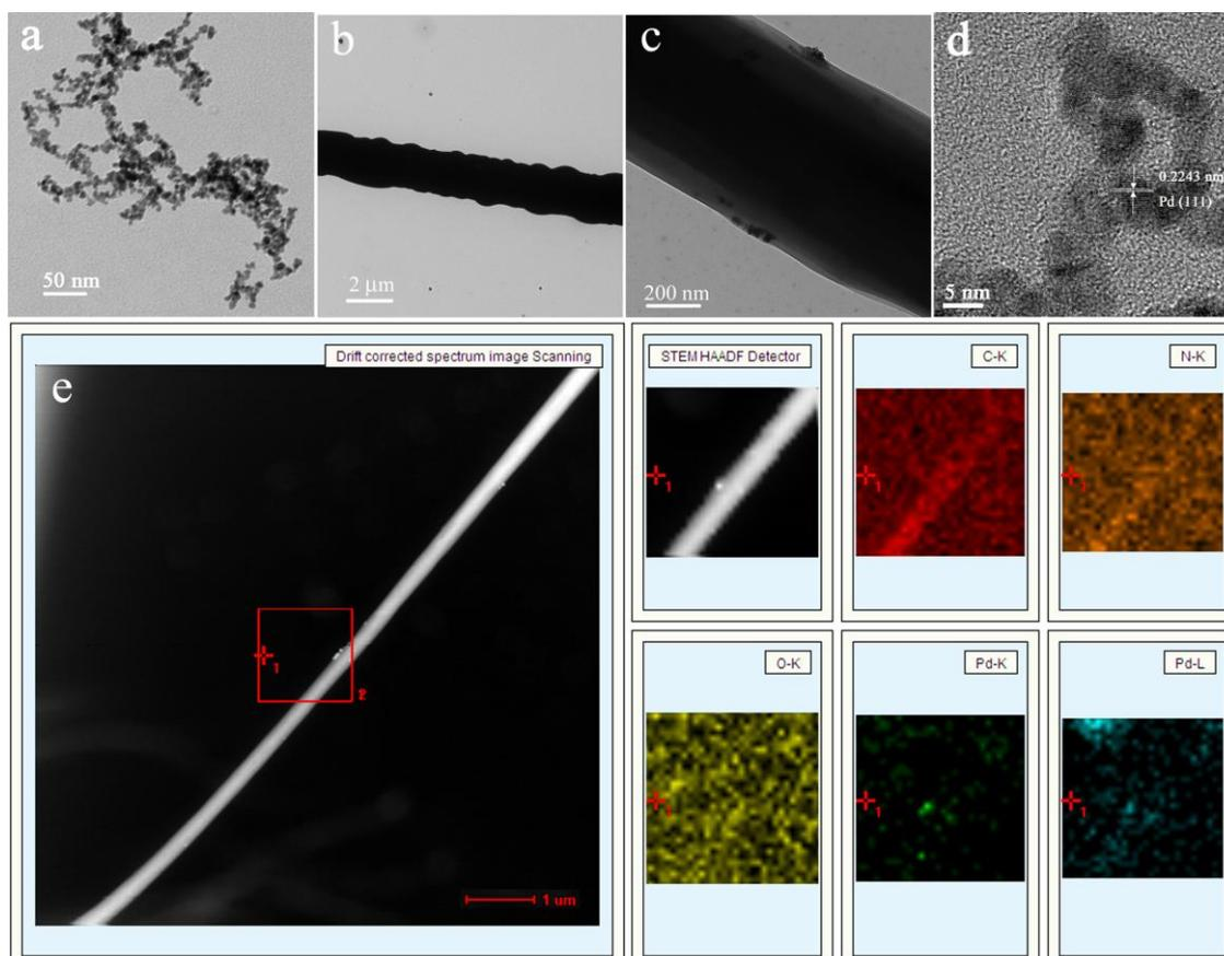
**Figure 3.** TEM images of the synthesized PdNPs (a), PEI/PCL fibers at 35:65 weight ratio (b) and modified with PdNPs (c), high resolution of PdNPs (d), and C/N/O/Pd elemental mapping (e) of PEI/PCL@PdNPs composites. The scale size of elemental mapping is 1.5  $\mu\text{m}$ .
