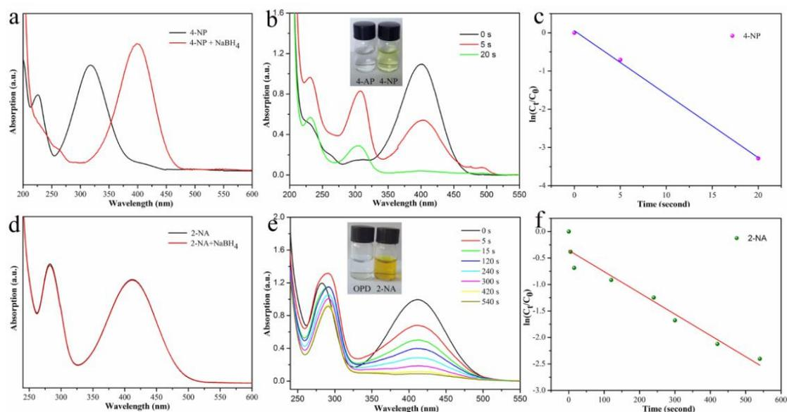
**Figure 8.** UV absorption curves of 4-NP and 2-NA before and after adding  $\text{NaBH}_4$  aqueous solution (a,d); catalytic reduction of 4-NP and 2-NA with PEI/PCL@PdNPs composite (PEI:PCL, w/w, 35:65) and photos of 4-NP and 2-NA solution after reduction (b,e); linear relationship of the reduction process (c,f).
