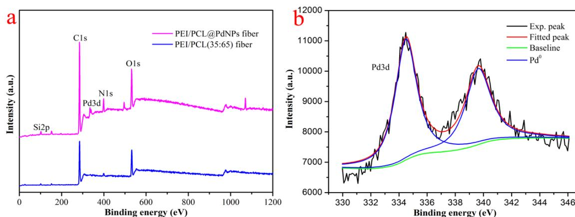
**Figure 7.** Survey X-ray photoelectron spectroscopy (XPS) spectra of the obtained PEI/PCL fiber and PEI/PCL@PdNPs (a) and deconvolutions of XPS peaks of the Pd3d region (b).
