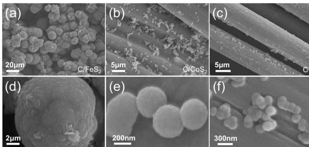
**Figure S2.** (a), (d) SEM images of C/FeS<sub>2</sub>; (b), (e) SEM images of C/CoS<sub>2</sub>; (c), (f) SEM images of C.
