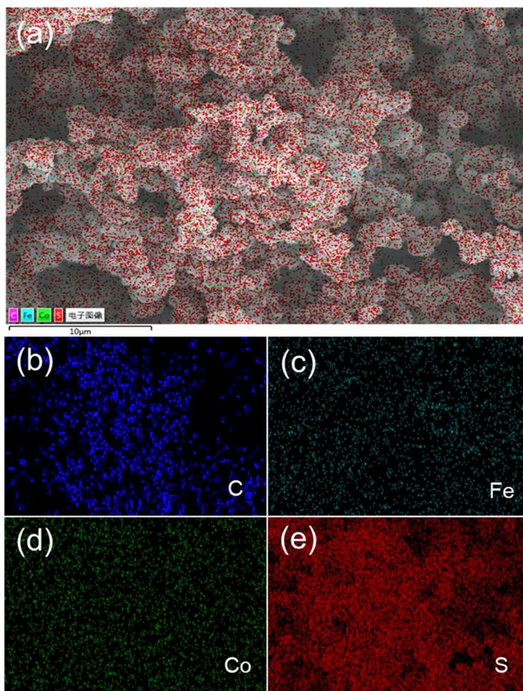
**Figure S1.** (a) SEM image of C/Co-FeS<sub>2</sub>/CoS<sub>2</sub>; (b-e) corresponding EDS elemental mapping images.
