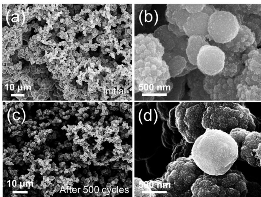
Figure S7. (a) and (b) SEM images of C/Co-FeS<sub>2</sub>/CoS<sub>2</sub>; (c) and (d) SEM images of C/Co-FeS<sub>2</sub>/CoS<sub>2</sub> after the 500 cycles.
