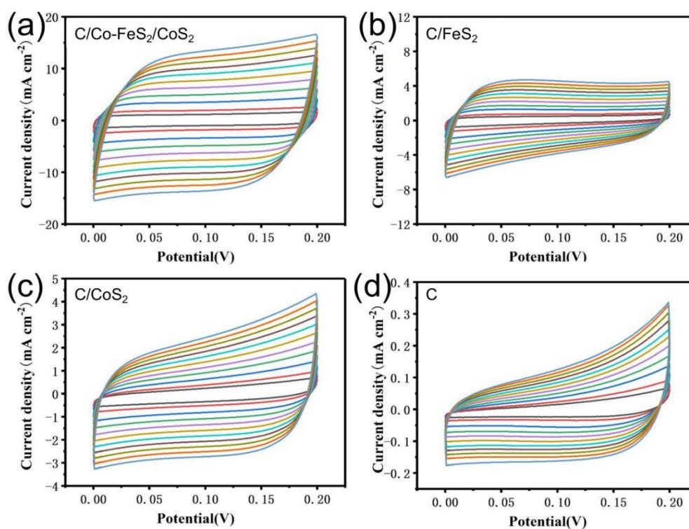
Figure S5. (a-d) cyclic voltammograms of C/Co-FeS<sub>2</sub>/CoS<sub>2</sub>, C/FeS<sub>2</sub>, C/CoS<sub>2</sub> and C were measured in the non-faradaic capacitance current range at scan rates of 5, 10, 20, 30, 40, 50, 60, 70, 80, 90 and 100 mV s<sup>-1</sup>.
