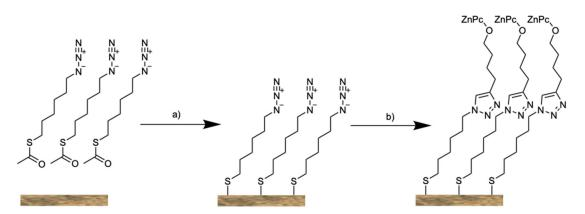
**Figure 2.** Schematic representation of the functionalization of npAu. (**a**) Formation of a self-assembled monolayer (SAM) using the azide functionalized acetyl protected thiol 1 followed by (**b**) "click chemistry" to bind the photosensitizer ZnPc 3.
