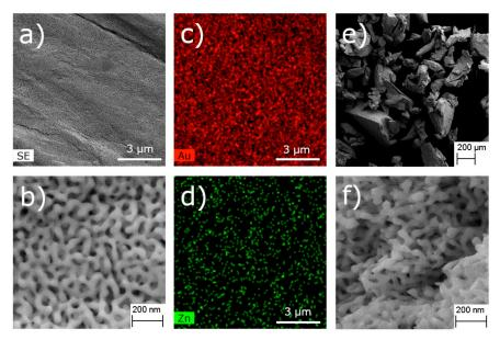
**Figure 3.** Structure of the npAu disk and powder after the two-step functionalization with the azide 1 without spacer and the photosensitizer ZnPc 3 (**a**) SEM image of the surface used for energy-dispersive X-ray (EDX) measurement, (**b**) SEM image of the porous structure with a magnification of 100,000, (**c**) EDX mapping for the element Au and (**d**) EDX mapping for the element Zn and SEM images of the structure of npAu powder with a magnification of (**e**) 10,000 and (**f**) 100,000.
