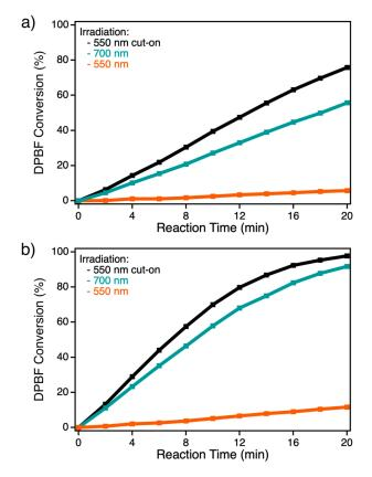
**Figure 5.** Photooxidation of DPBF at different irradiation wavelengths irradiating only the ZnPc absorption using a 700 nm filter (cyan), only the npAu plasmon resonance using a 550 nm filter (orange) or both absorption sites simultaneously using a 550 nm cut-on filter (black) and (**a**) a ZnPc functionalized npAu disk or (**b**) a ZnPc functionalized npAu powder as hybrid photocatalyst.
