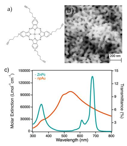
**Figure 1.** Structure of (**a**) the photosensitizer zinc phthalocyanine 3 used in this study, (**b**) porous structure of npAu and (**c**) corresponding optical spectra for zinc (II) phthalocyanine (ZnPc) (cyan) and transmission spectrum of a nanoporous gold foil with a thickness of 100 nm (orange) prepared as described in [20].
