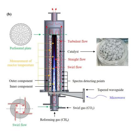
**Figure 9.** (a) Flow diagram and (b) schematic diagrams of the experimental setup of microwave plasma–catalytic reactor used for syngas production.
