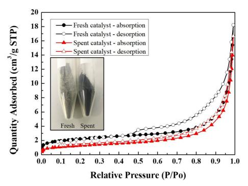
Figure 4. Adsorption–desorption isotherms of N<sub>2</sub> at 77K for the fresh and spent catalysts.
