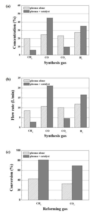
Figure 6. (a) Concentration, (b) flow rate, and (c) conversion ratio obtained with different reforming methods.
