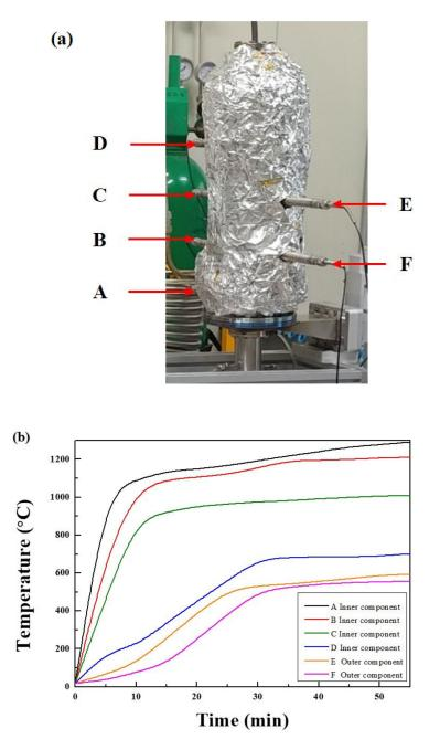
**Figure 3.** (a) Photograph of the insulated outer surface of the microwave plasma–catalytic reactor. (b) Temperature changes in the inner and outer components measured over 1 h using various thermocouples.
