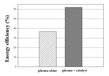
Figure 8. Energy efficiency of dry reforming obtained using the hybrid system.
