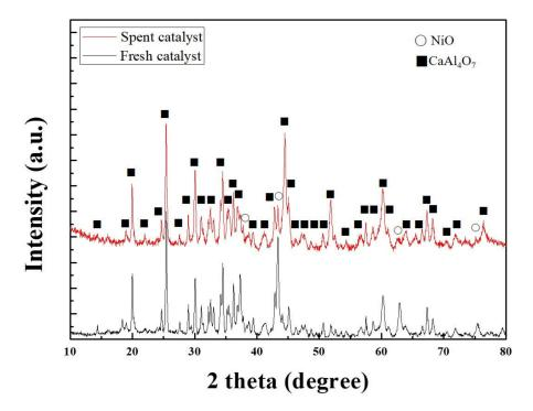
Figure 5. Powder X-ray diffraction (XRD) patterns of the fresh and spent catalysts.
